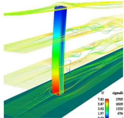
Figure : Deformation of a cantilever subject to a uniform flow, Hrvoje Jasak ©
