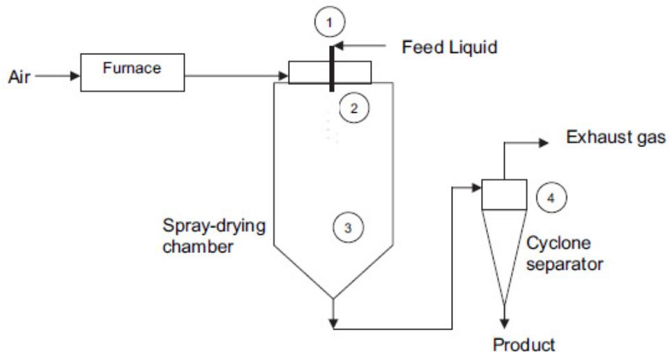
Figure 2.2: The process stages of spray drying [52].
