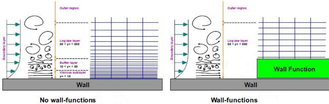
Figure 7.6: Different near-wall treatments [54].
