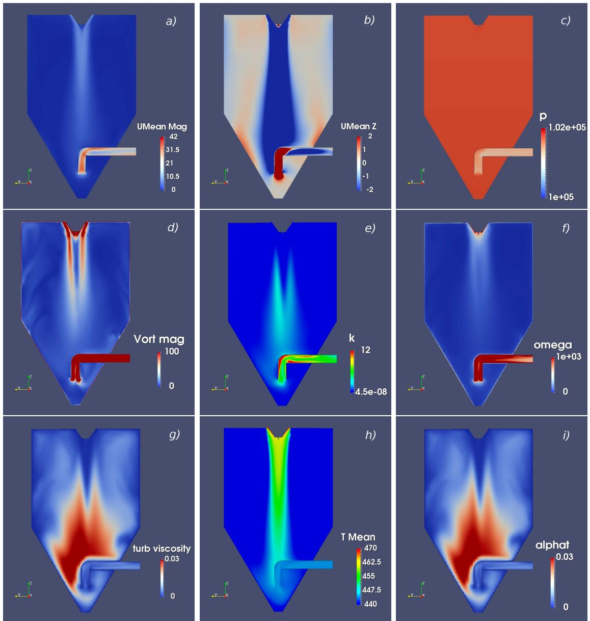
Figure 9.4.6: Color plots for the case with heat transfer. Please, note that in picture i) "alphat" means the turbulent diffusivity  $\alpha_T$ , and also in picture f) "omega" means the specific turbulent dissipation  $\omega$ . Regarding the other figures see caption of Figure 9.2.2.
