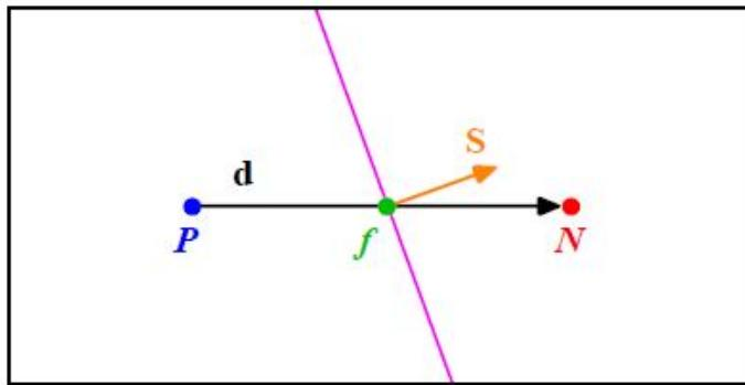
Figure 7.1: Mesh orthogonality [54].
