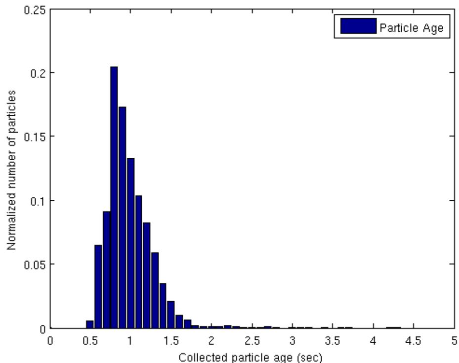
Figure 9.5.7: Solid case - 20'000 part/sec - Distribution of collected particles age normalized by the total number of collected particles.
