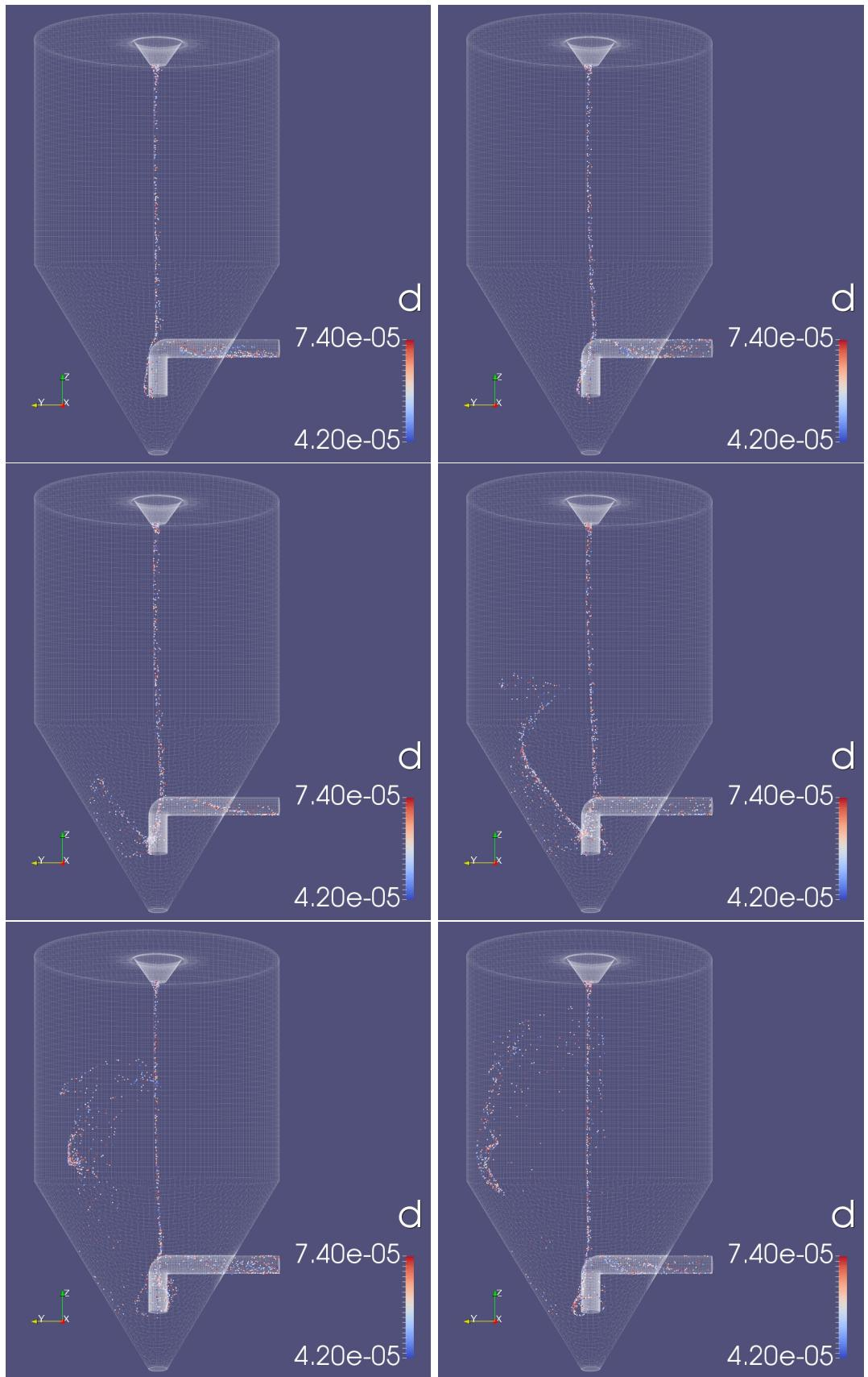
Figure 9.5.12: Second class of particle diameters as a function of time: 1.5s on the top left - 2.5 on the top right - 3.5s on the middle left - 4.5s on the middle right - 5.5s on the bottom left - 6.5s on the bottom right.
