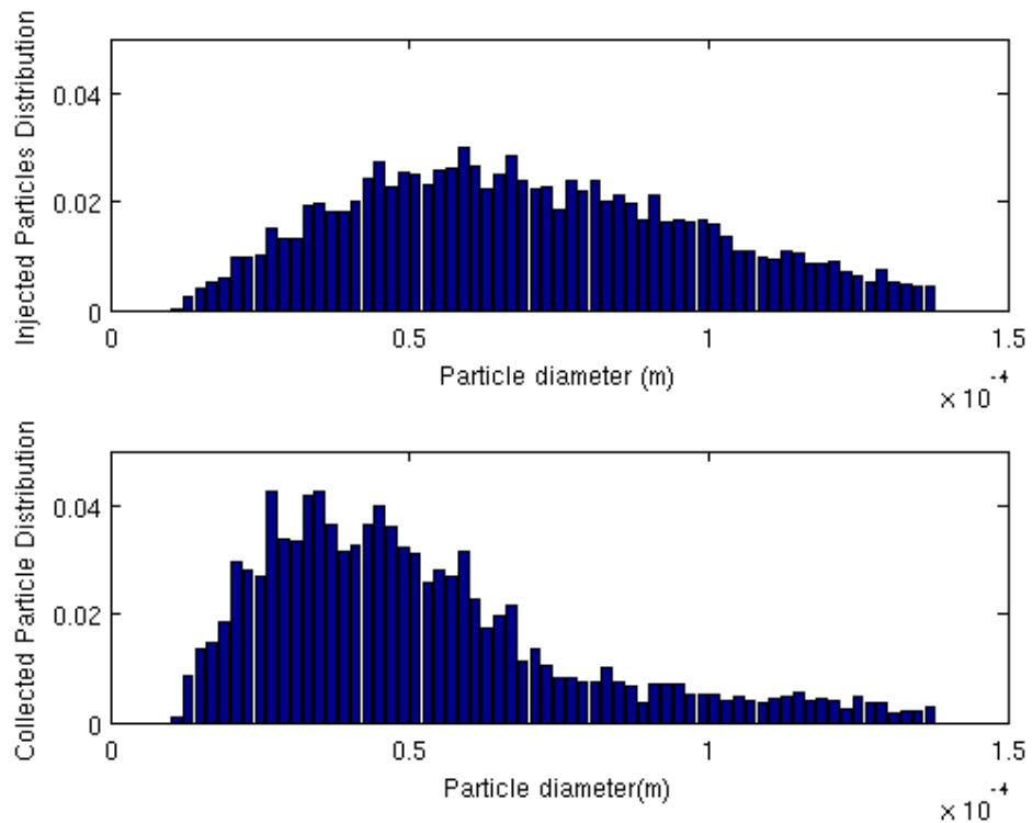
Figure 9.5.8: Solid case - 20'000 part/sec - Injected particles distribution normalized by the sum of the injected particles - on the top. Collected particles distribution normalized by the sum of the collected particles - on the bottom.
