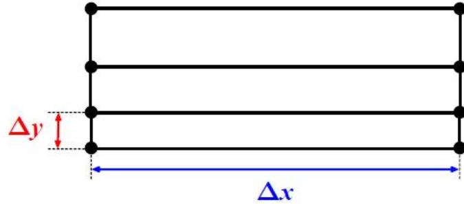
Figure 7.3: Mesh aspect ratio [54].
