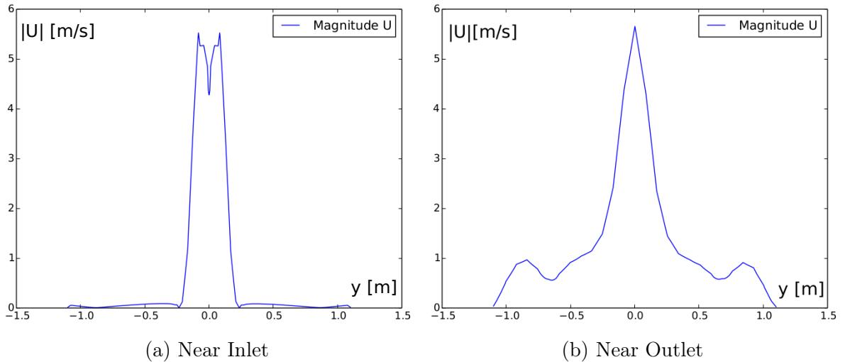
Figure 9.3.1: Velocity magnitude profiles calculated with SST $k-\omega$  model.
