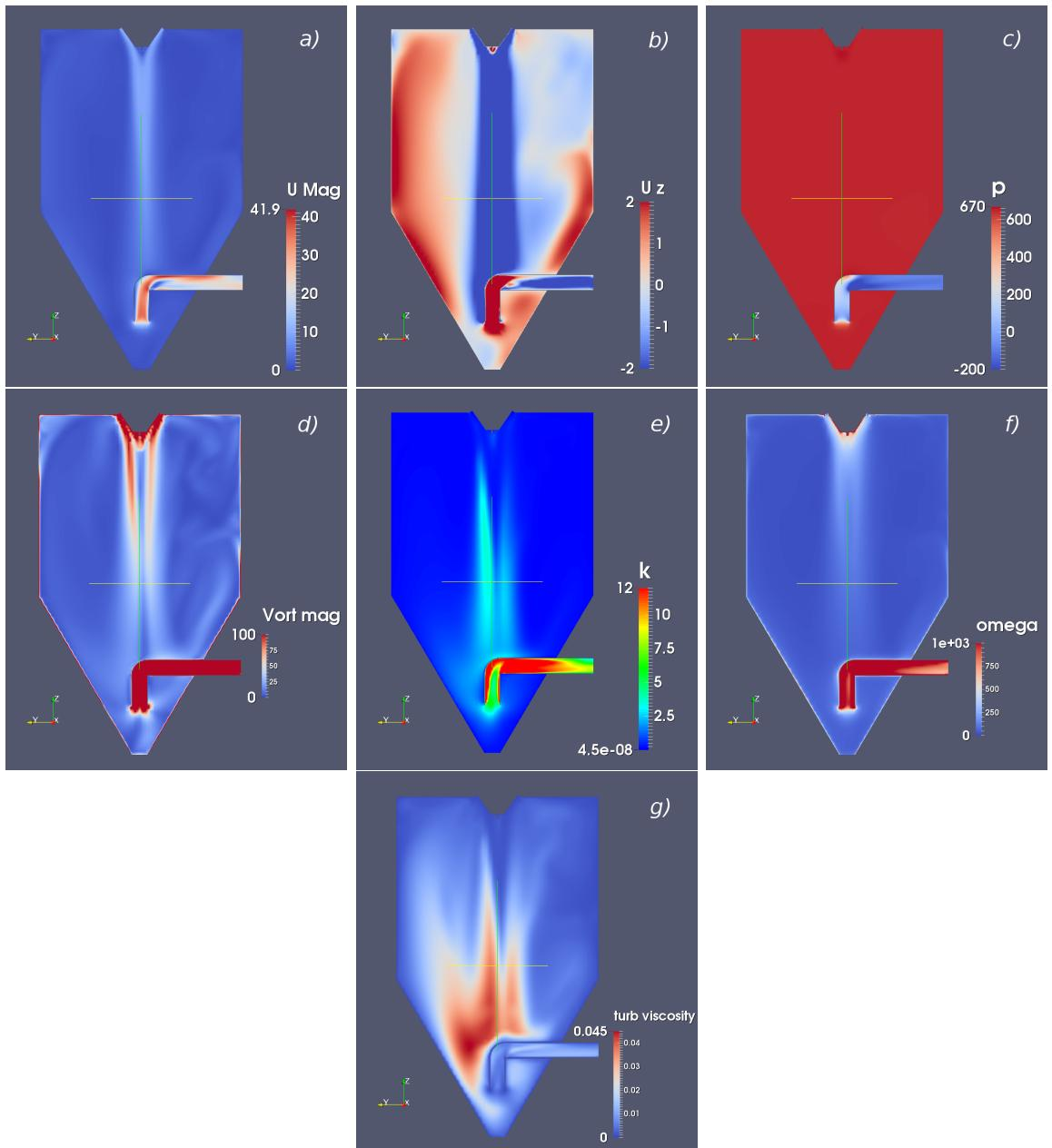
Figure 9.2.2: Overview of the results of each calculated variable for case C. a) the magnitude of the velocity  $U$  - b)  $z$  velocity component  $U_z$ ; it is the most relevant one - c) pressure  $p$  - d) the magnitude of the vorticity  $Z$  - e) the turbulent kinetic energy  $k$  - f) the specific turbulent dissipation  $\omega$  - g) the turbulent viscosity  $\nu_T$
