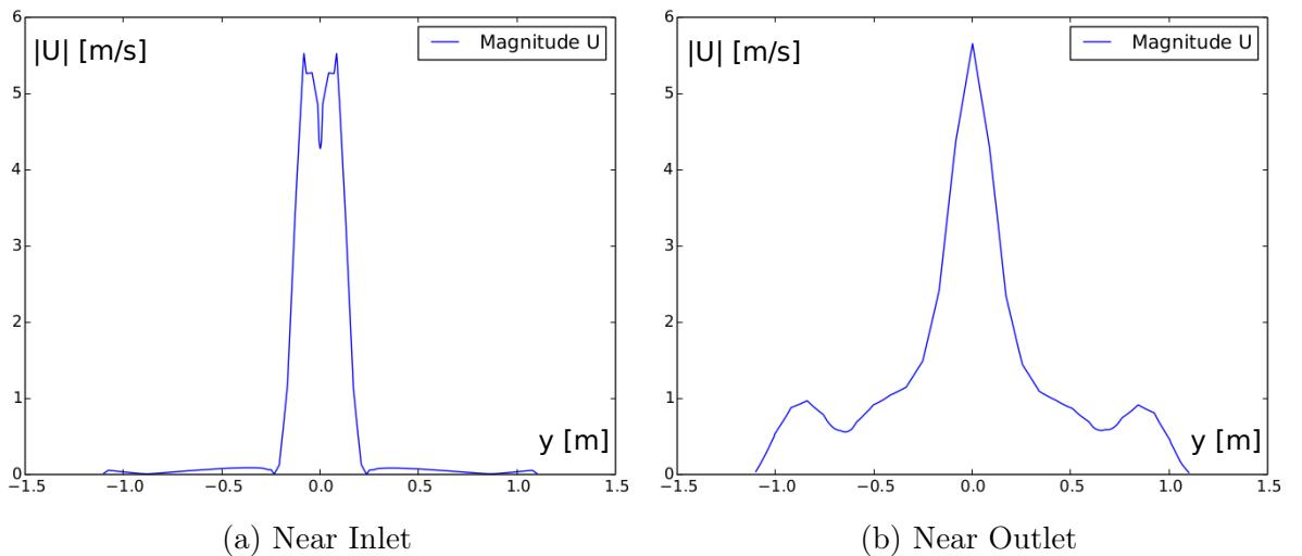
Figure 9.3.2: Velocity magnitude profiles calculated with  $k-\epsilon$  model.
