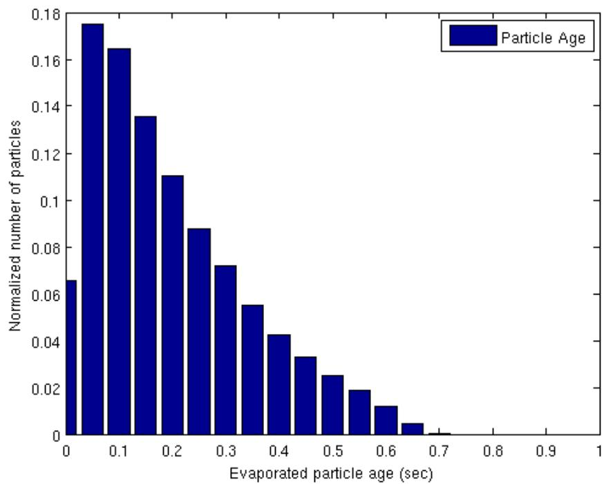
Figure 9.5.4: Liquid case - 20'000 part/sec - Distribution of the evaporated particles age normalized by the total number of evaporated particles.
