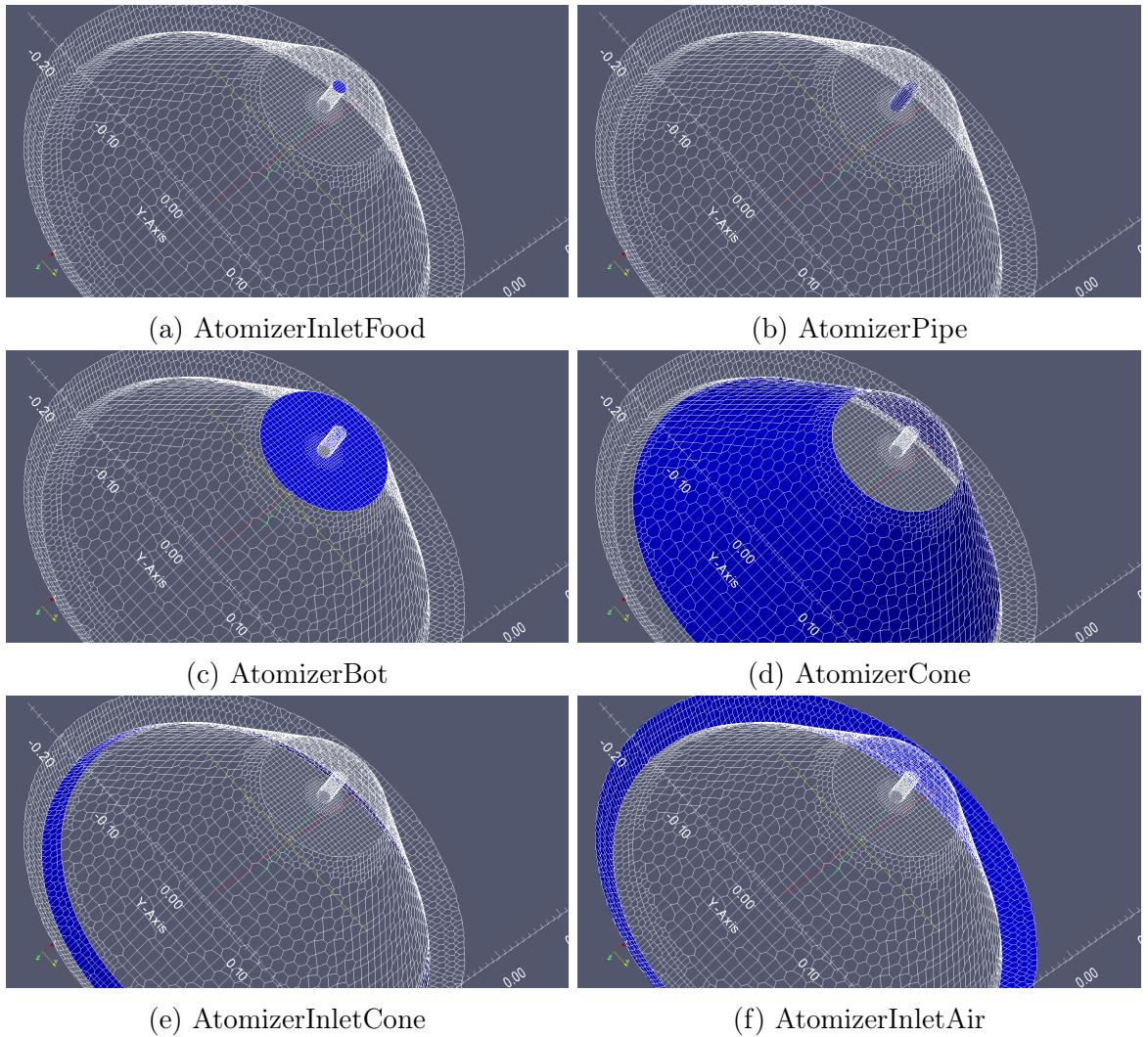
Figure 6.2.3: Different parts of the atomizer.
