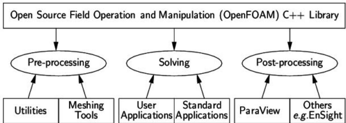
Figure 4.1: Overview of OpenFOAM structure [48].
