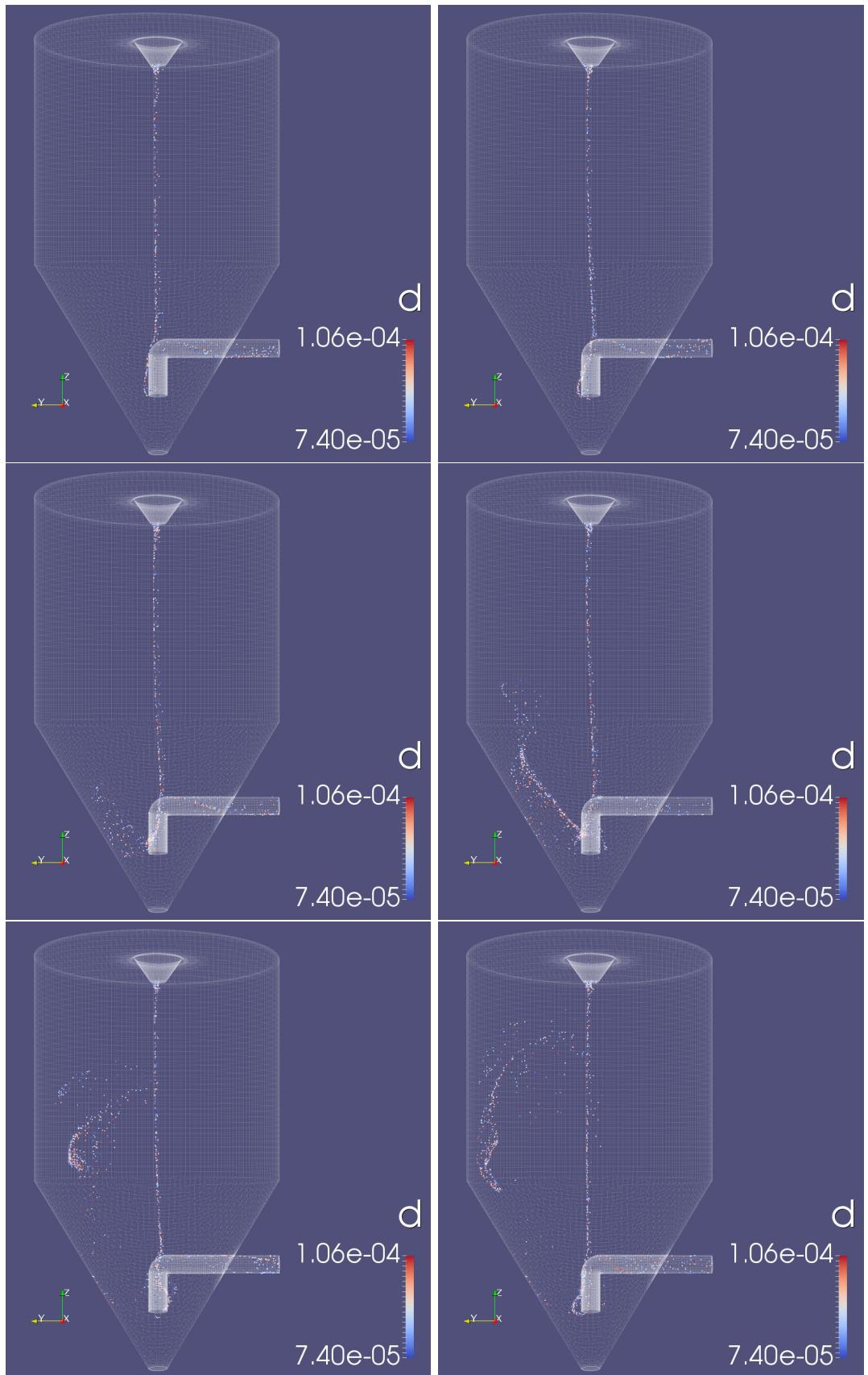
Figure 9.5.13: Third class of particle diameters as a function of time: 1.5s on the top left - 2.5 on the top right - 3.5s on the middle left - 4.5s on the middle right - 5.5s on the bottom left - 6.5s on the bottom right.
