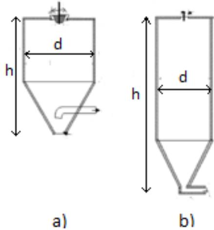
Figure 2.1: Spray dryer short-form a) and tall-form b) [23].
