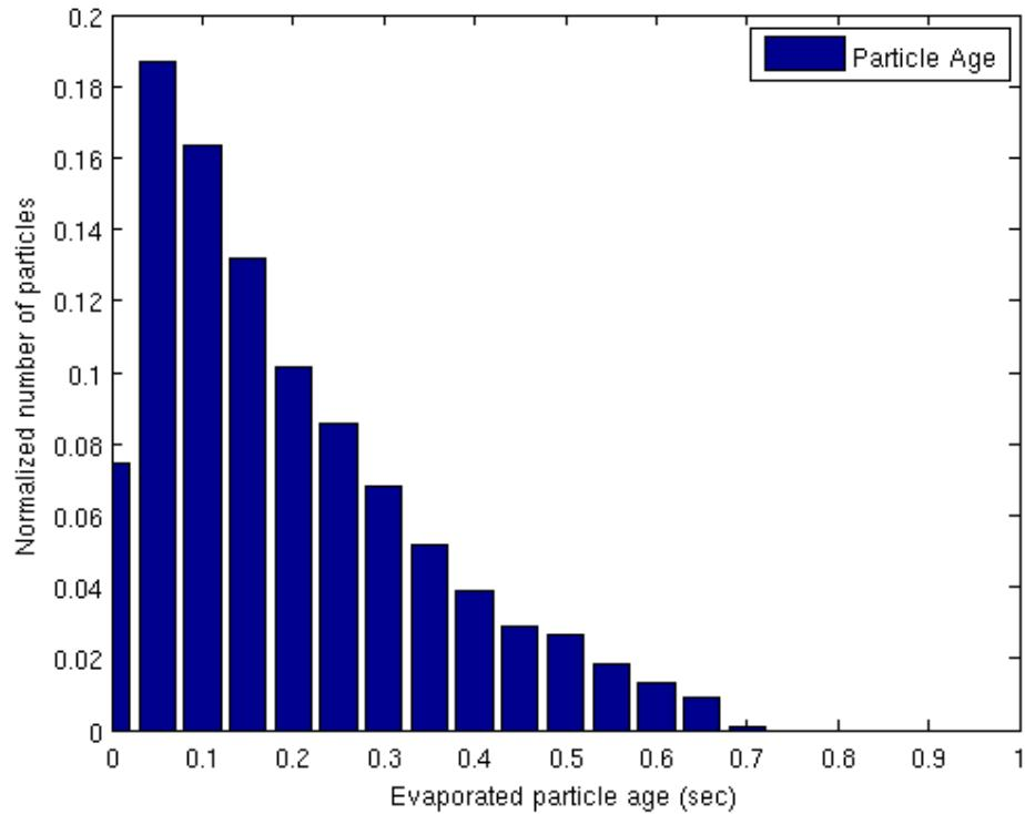
Figure 9.5.1: Liquid case - 2'000 part/sec - Distribution of the evaporated particles age normalized by the total number of evaporated particles.
