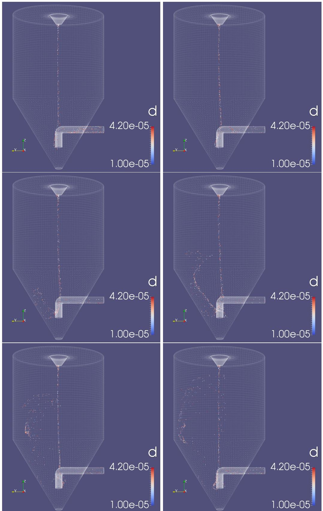
Figure 9.5.11: First class of particle diameters as a function of time: 1.5s on the top left - 2.5 on the top right - 3.5s on the middle left - 4.5s on the middle right - 5.5s on the bottom left - 6.5s on the bottom right.
