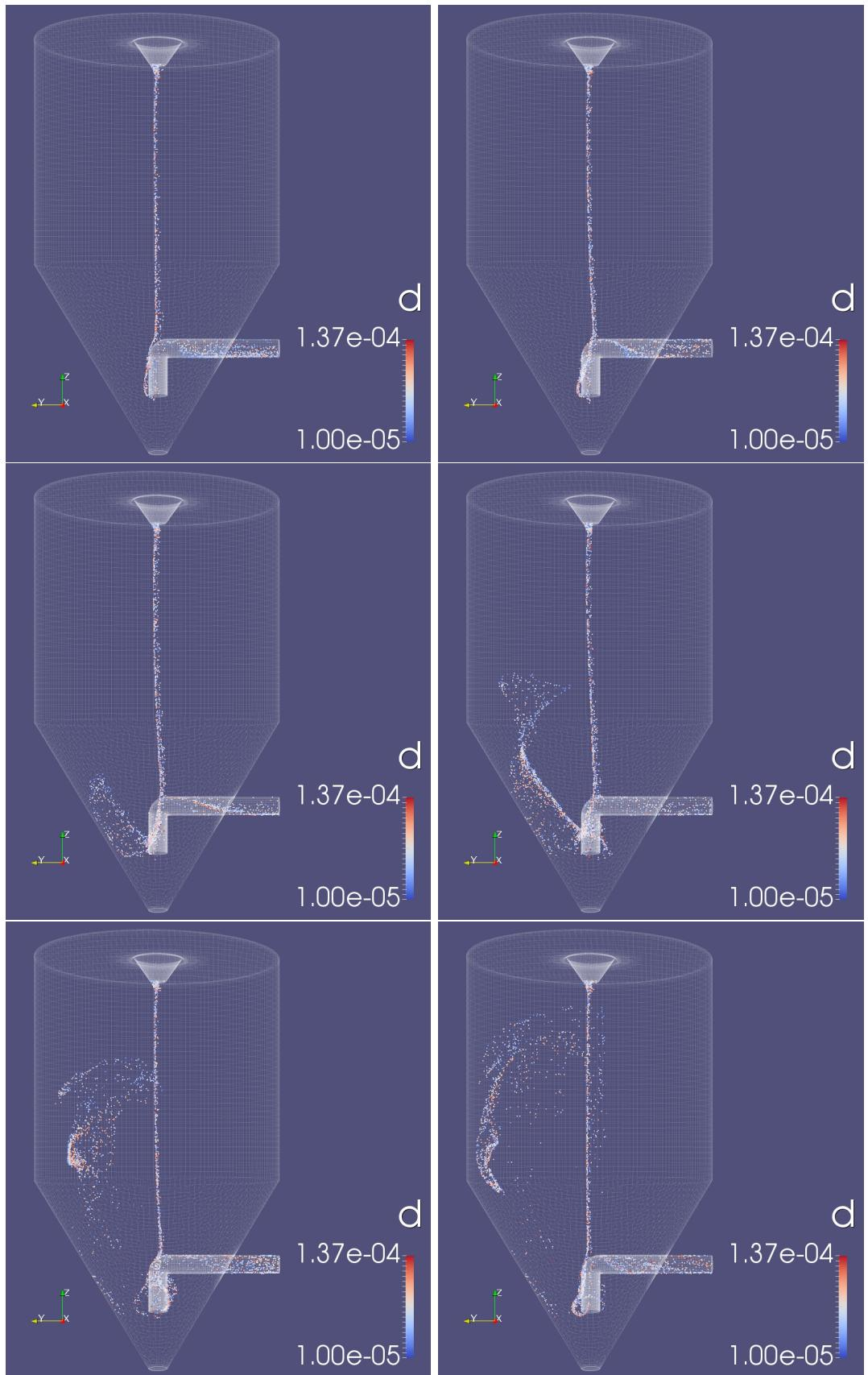
Figure 9.5.10: Total range of particles as a function of time: 1.5s on the top left - 2.5s on the top right - 3.5s on the middle left - 4.5s on the middle right - 5.5s on the bottom left - 6.5s on the bottom right.
