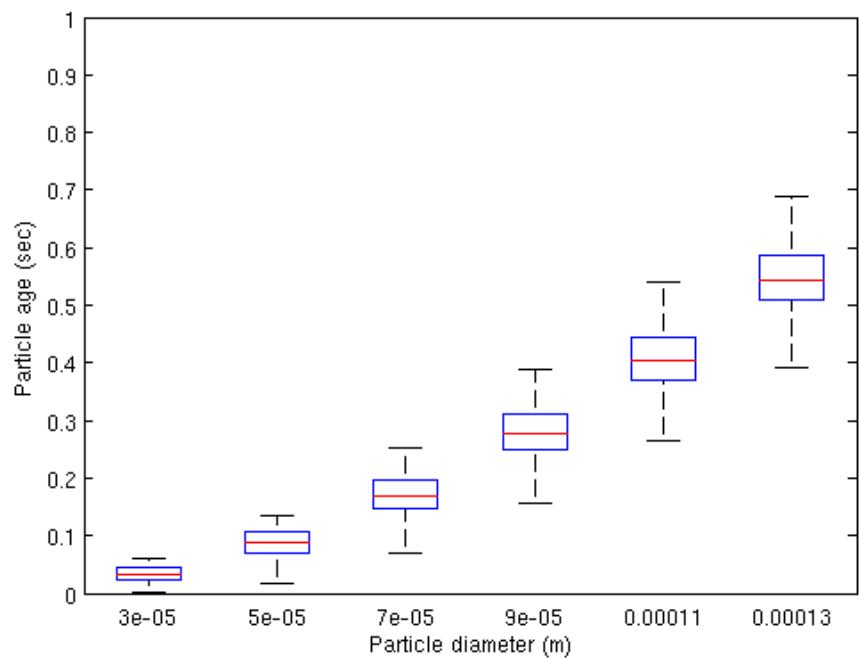
Figure 9.5.5: Liquid case - 20'000 part/sec - Particle age divided in diameter classes.
