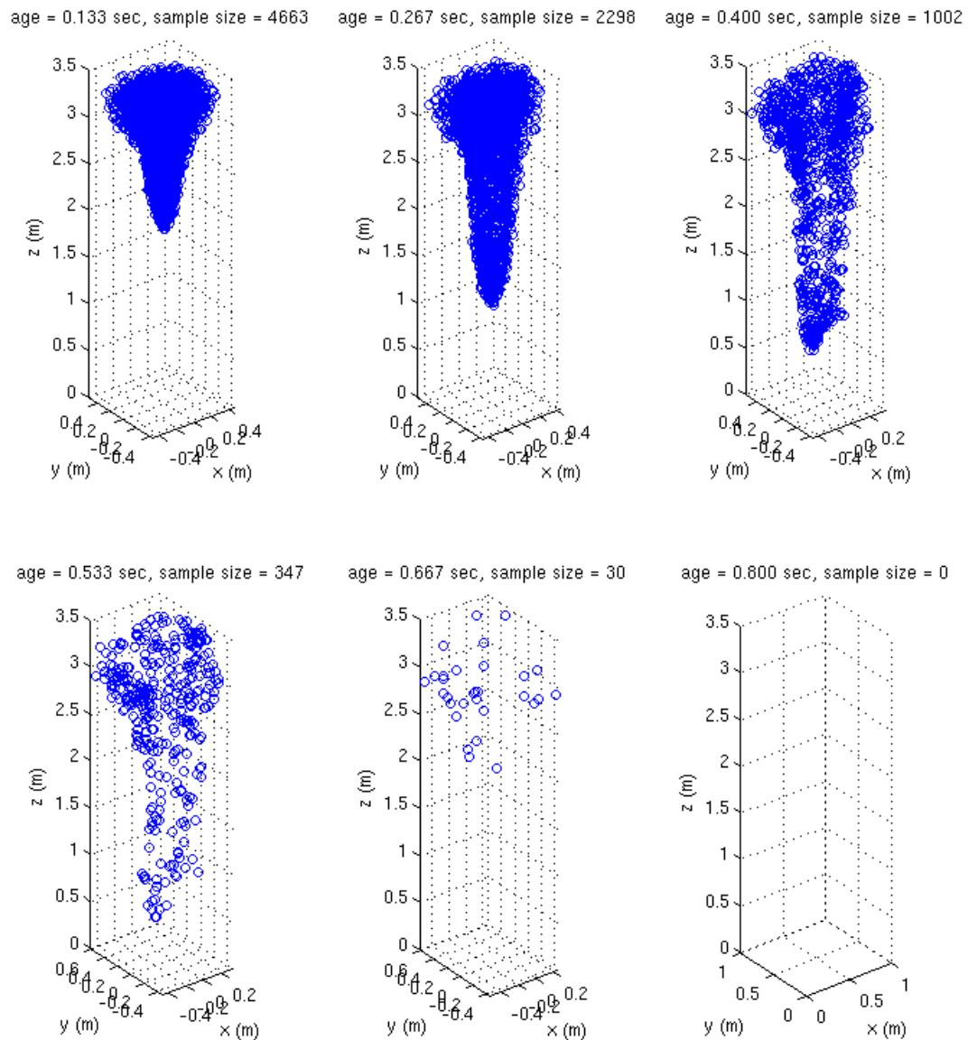
Figure 9.5.3: Liquid case - 2'000 part/sec - Spatial distribution of the evaporated particles.
