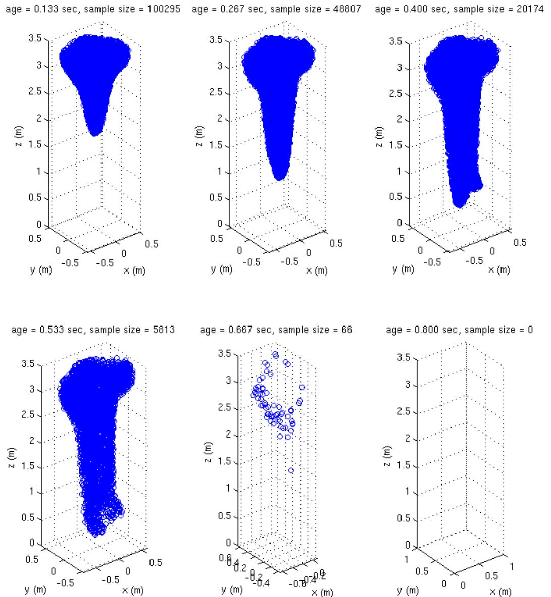
Figure 9.5.6: Liquid case - 20'000 part/sec - Spatial distribution of the evaporated particles.
