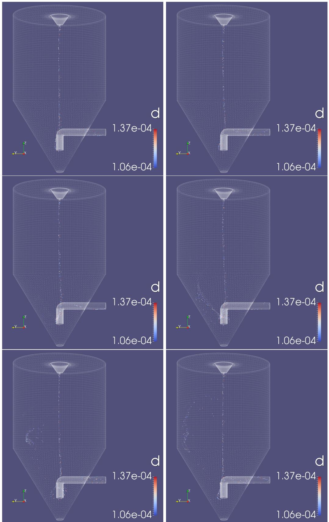
Figure 9.5.14: Fourth class of particle diameters as a function of time: 1.5s on the top left - 2.5 on the top right - 3.5s on the middle left - 4.5s on the middle right - 5.5s on the bottom left - 6.5s on the bottom right.
