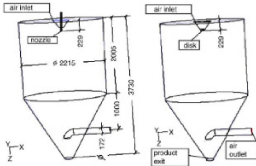
Figure 6.1.2: Huang's geometry [7].
