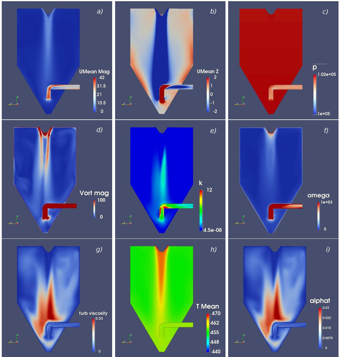
Figure 9.4.5: Color plots the adiabatic case. Please, note that in picture *i*) "alphat" means the turbulent diffusivity  $\alpha_T$ , and also in picture *f*) "omega" means the specific turbulent dissipation  $\omega$ . Regarding the other figures see caption of Figure 9.2.2.
