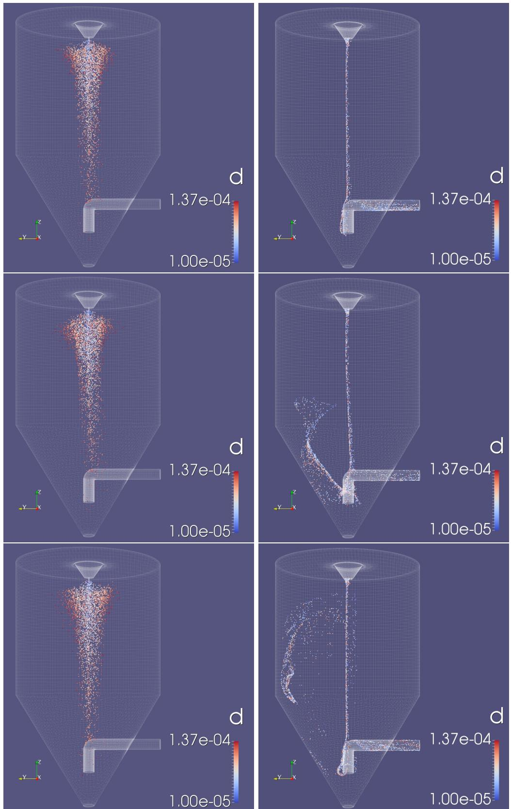
Figure 9.5.15: Comparison between liquid and solid phase. Images in left columns represent liquid phase, while those in right columns represent solid phase. Figures on the top represent instant  $t=1.5\text{s}$ , those in the middle  $t=4.5\text{s}$  and those on the bottom  $t=6.5\text{s}$ .
