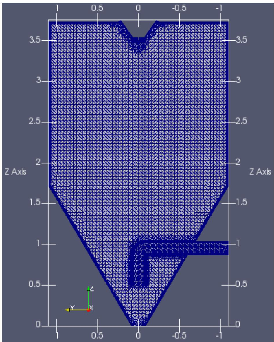
Figure 7.7: snappyHexMesh refinement.
