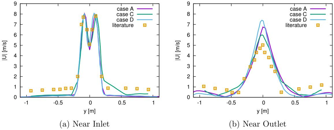
Figure 9.2.1: Velocity magnitude profiles for different cases.
