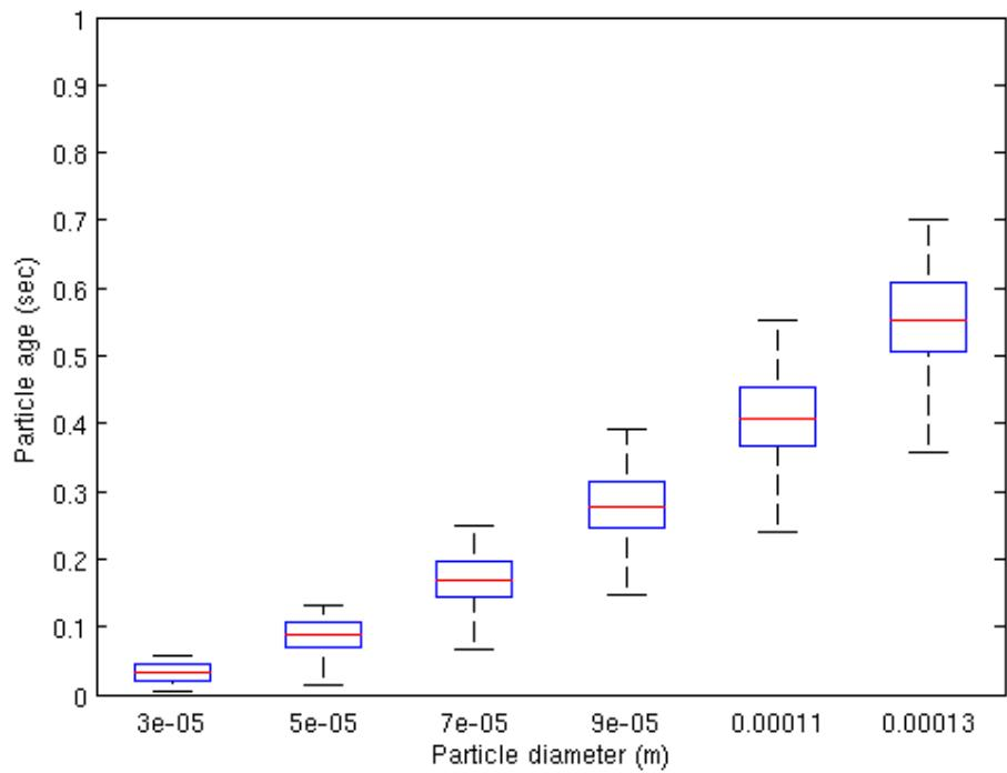
Figure 9.5.2: Liquid case - 2'000 part/sec - Particle age divided in diameter classes.
