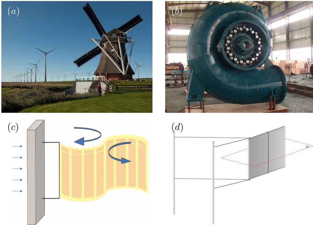
Figure 7.3.2: Traditional windmill in front of a modern wind farm (a), Francis turbine for hydroelectric power generation (b) and schematics of the water-eel and of the flapping wing energy harvesters (c-d).
