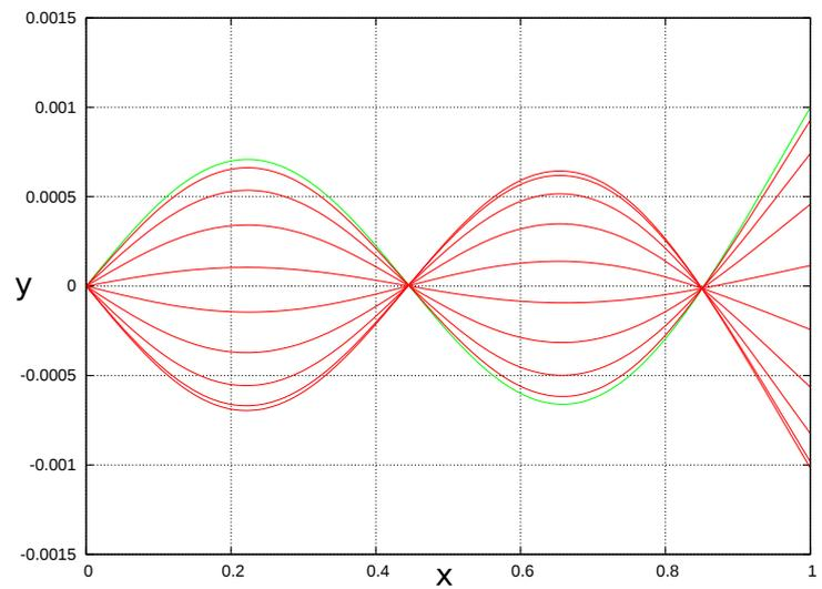
Figure 6.5.14: Beam snapshots during one oscillation. Initial condition (in green) is such that only the third oscillation mode of the hinged beam is excited.
