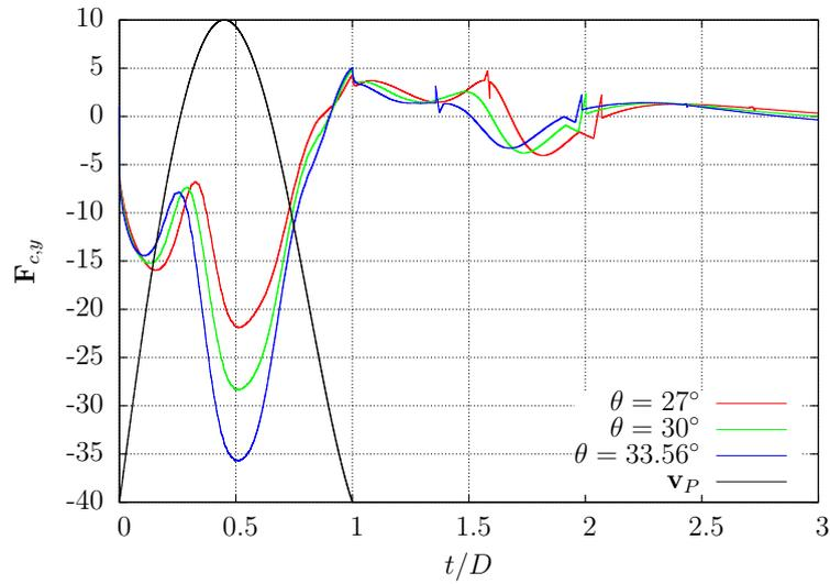
Figure 7.2.10: Time history of the y-force component acting at the attachment point of the filament for different filament angles. The velocity of the plate is in black.
