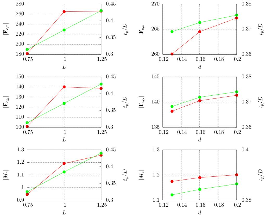
Figure 7.2.20: Peak values of force  $|\mathbf{F}_c|$  and moment  $|M_c|$  (in red) and corresponding time (in green) for the right filament in the “hole” case. The left column shows the values for different filament length  $L$ , while in the right column the inter-tip distance  $d$  varies.
