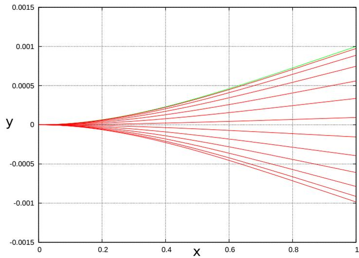
Figure 6.5.10: Beam snapshots during one oscillation. Initial condition (in green) is such that only the first oscillation mode of the clamped beam is excited.
