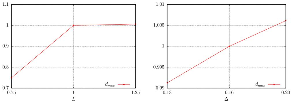
Figure 7.2.50: Maximum values of the tendency to detach  $d$  for the hole case for different filament lengths  $L$  and  $\Delta = 1.6$  (left), and for different  $\Delta$  and  $L = 1$  (right).
