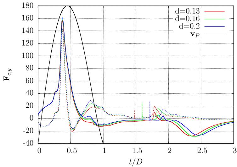
Figure 7.2.18: Time history of the y-force component acting at the attachment point of the right (line) and left (dots) filament for different inter-tip distances. The velocity of the plate is in black.
