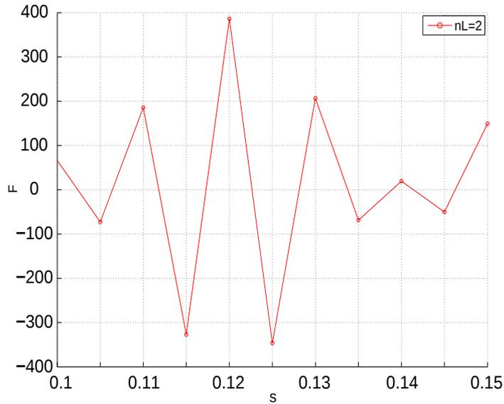
Figure 5.4.1: Lagrangian forces  $\mathbf{F}$  along the curvilinear abscissa  $s$  of a simply hinged filament subject to an incoming flow. In this simulation 2 Lagrangian points per Eulerian grid were approximately used to describe the surface.
