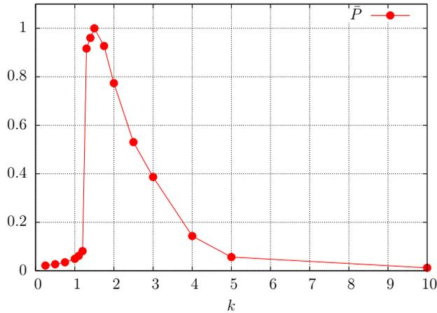
Figure 7.3.11: Mean extracted power  $\bar{P}$  as a function of the spring stiffness  $k$  for  $Re = 200$ . The peak value is found for  $k = 1.5$ .
