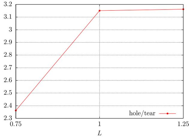
Figure 7.2.44: Ratio between the maximum tendency to detachment between the hole and tear configuration for different filament lengths  $L$  and  $\theta = 33.56^\circ$ .
