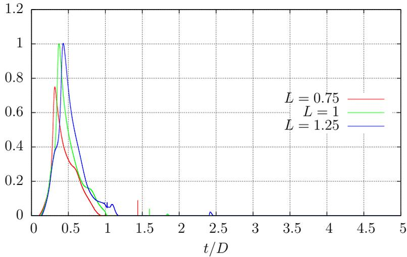
Figure 7.2.49: Tendency to detachment for the hole case (left filament) with different inter-tip distance and  $L = 1$ . Results have been scaled with the maximum tendency to detachment in time for  $d = 1.6$ .
