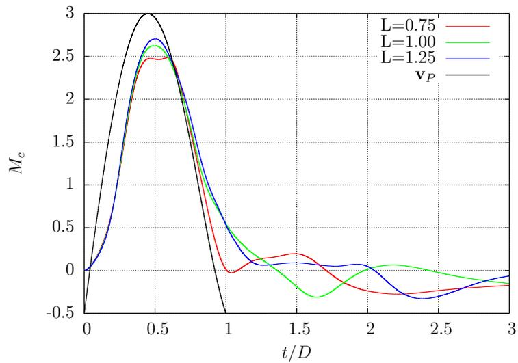
Figure 7.2.8: Time history of the moment acting at the attachment point of the filament for different filament lengths. The velocity of the plate is in black.
