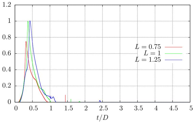
Figure 7.2.48: Tendency to detachment for the hole case (left filament) with different lengths and inter-tip distance equal to  $1.6$ . Results have been scaled with the maximum tendency to detachment in time for  $L = 1$ .
