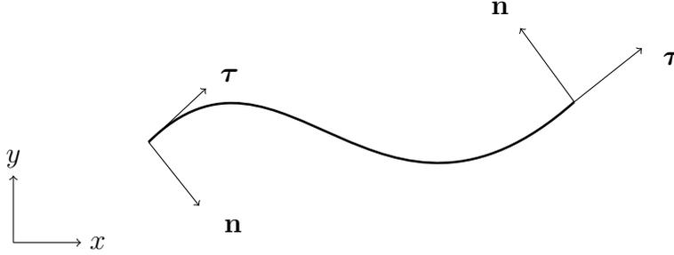
Figure 3.3.2: Local tangential  $\boldsymbol{\tau}$  and normal  $\mathbf{n}$  unit vectors. By definition  $N$  and  $T$  reactions are aligned with these vectors.
