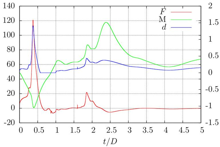
Figure 7.2.40: Punctual loads ( $F$ ,  $M$ , on the left) and tendency to detachment ( $d$ , on the right) in the hole case, right filament (scaled with the maximum tendency to detachment in time for the tear configuration).
