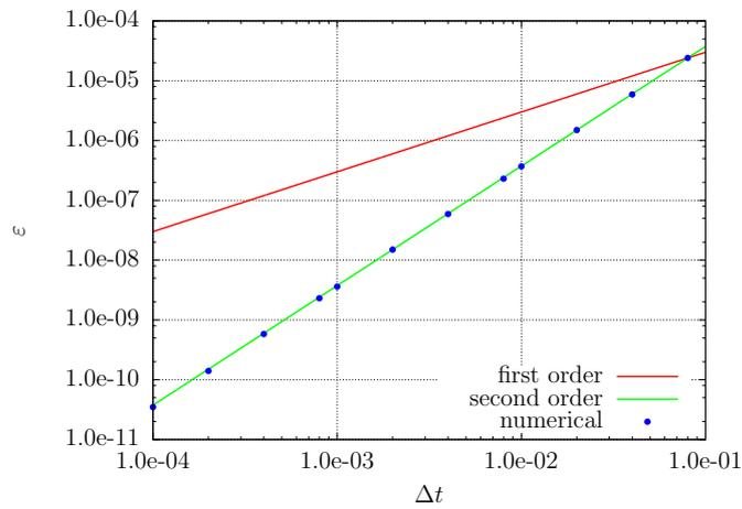
Figure 6.5.1: Temporal convergence rate of the numerical code (dots) compared with the theoretical first- and second-order error curves.
