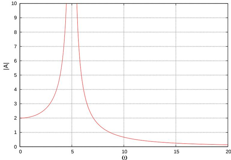
Figure 3.1.3: Theoretical oscillation amplitude magnitude as a function of the imposed driving force frequency  $\omega_F$ . The peak in correspondence of natural frequency  $\omega_N$  is clearly visible.
