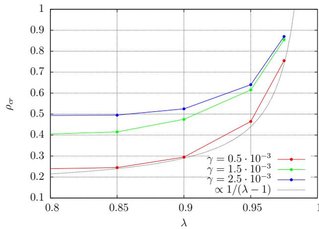
Figure 7.1.6: Critical value of  $\rho$  with  $\lambda$  for different values of bending stiffness  $\gamma$ .
