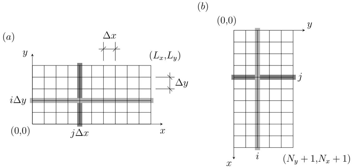
Figure 6.4.1: Computational domain (a) and data field storage in matrix form (b), where  $L_x = N_x \Delta x$ ,  $L_y = N_y \Delta y$ .
