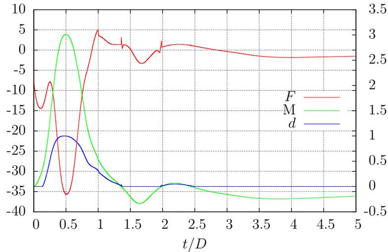
Figure 7.2.38: Punctual loads ( $F$ ,  $M$ , on the left) and tendency to detachment ( $d$ , on the right) in the tear case (normalized to 1 as the reference case).
