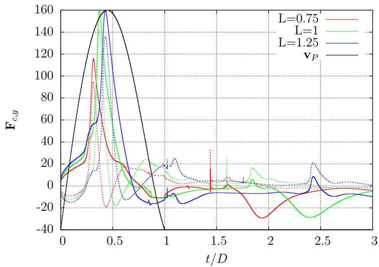
Figure 7.2.15: Time history of the y-force component acting at the attachment point of the right (line) and left (dots) filament for different filament lengths. The velocity of the plate is in black.
