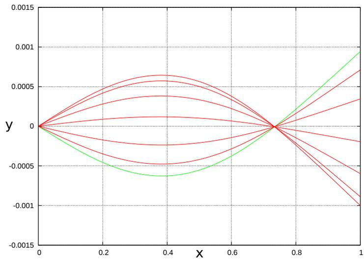
Figure 6.5.13: Beam snapshots during one oscillation. Initial condition (in green) is such that only the second oscillation of the hinged beam mode is excited.
