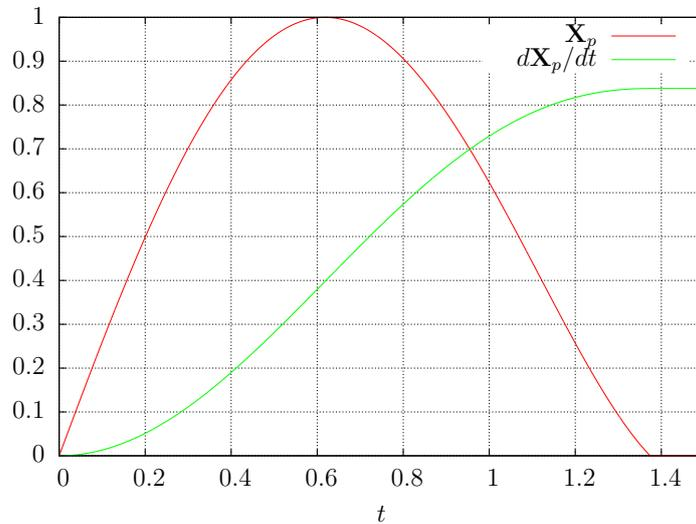
Figure 7.2.3: Plate position  $\mathbf{X}_p = r\theta$  (red) and velocity  $d\mathbf{X}_p/dt = r d\theta/dt$  (green) as function of time (Figure 7.2.4).
