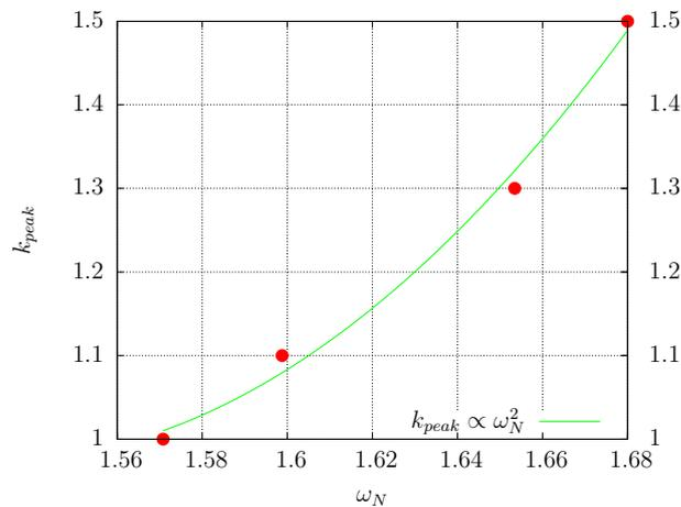
Figure 7.3.9: Relation between the natural oscillation pulsatance  $\omega_N$  and the optimal spring stiffness  $k_{peak}$  as predicted by equation (7.3.1).
