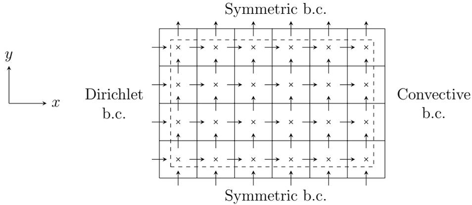
Figure 6.2.1: Staggered grid with applied boundary conditions (b). The dashed line encloses the computational domain.
