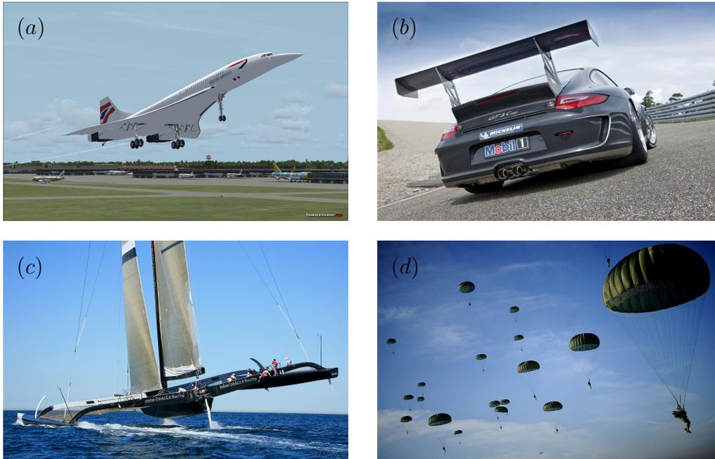
Figure 2.1.1: Examples of aerodynamical forces in action: in (a) the airplane takes off thanks to the lift forces generated on its wings, in (b) the down-force on the spoiler helps the car adhere to the pavement, in (c) hydrofoils contribute in raising the trimaran hulls out of the water, while in (d) drag force helps the parachutist reaching a limited terminal falling velocity.
