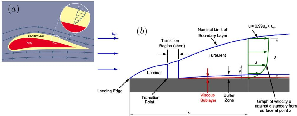
Figure 2.1.3: Schematic of boundary layer (in yellow) around a solid object (a), and boundary layer growing over a flat plate (b) with different regimes of flow (not in scale).
