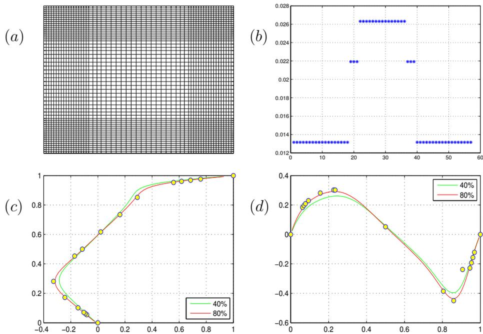
Figure 6.5.5: Stretched grid used for the simulation (a) and grid steps distribution along  $x$  (b).  $u$  (c) and  $v$  (d) velocity profiles at, respectively,  $x = 0.5$  and  $y = 0.5$  for different percentage of sliding wall velocity profile (Eq. (6.5.2)). Dots in (c) and (b) represent the profiles simulated in [88].
