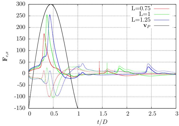
Figure 7.2.14: Time history of the x-force component acting at the attachment point of the right (line) and left (dots) filament for different filament lengths. The velocity of the plate is in black.
