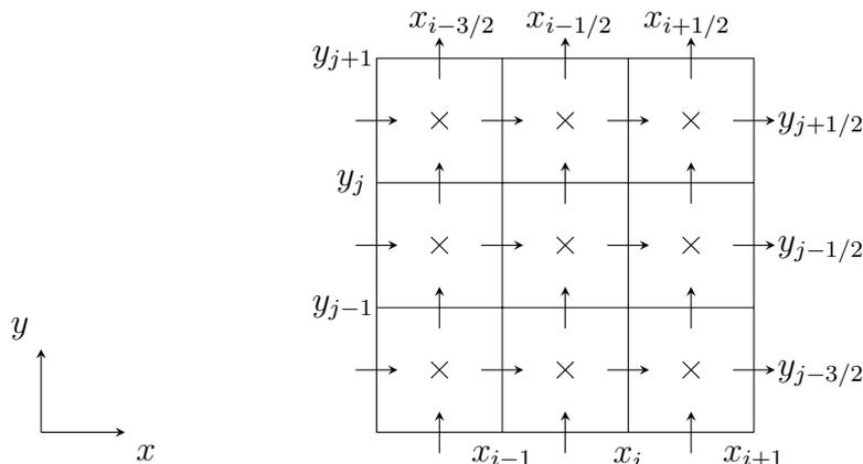
Figure 6.1.1: Staggered grid. x-velocity component  $u_x$  is evaluated at  $\rightarrow$ , y-velocity component  $u_y$  at  $\uparrow$ , whereas pressure at  $\times$ .
