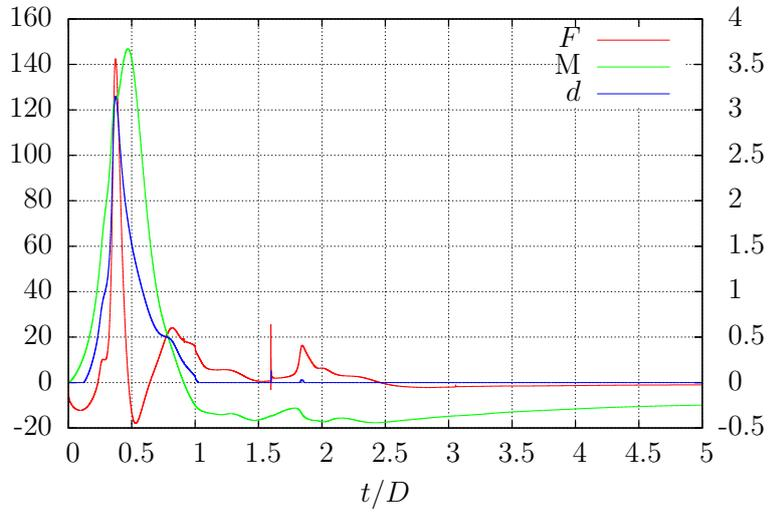
Figure 7.2.39: Punctual loads ( $F$ ,  $M$ , on the left) and tendency to detachment ( $d$ , on the right) in the hole case, left filament (scaled with the maximum tendency to detachment in time for the tear configuration).
