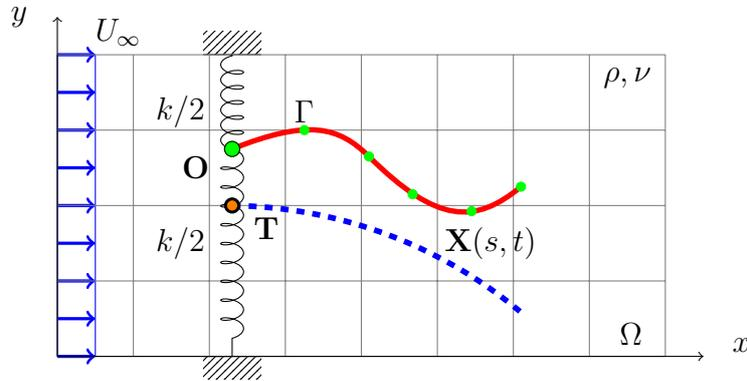
Figure 7.3.3: Filament  $\Gamma$  is hinged (initial condition in dashed blue line) to point  $\mathbf{O}$ , constrained to move only in vertical direction and linked by two springs of stiffness  $k/2$  to external fixed boundaries (not considered in the flow simulations).
