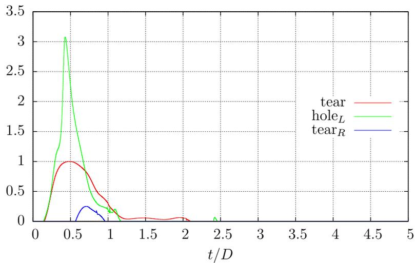
Figure 7.2.43: Tendency to detachment for the tear and hole case (right and left filaments) scaled with the maximum tendency to detachment in time for the tear configuration. Simulations for  $L = 1.25$  and  $\theta = 33.56^\circ$ .
