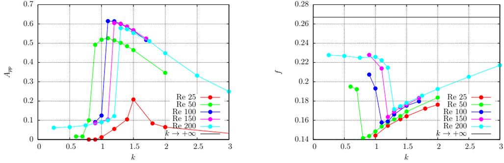
Figure 7.3.7: Flapping peak-to-peak amplitude (left) and frequency (right) of the leading edge for different Reynolds numbers.
