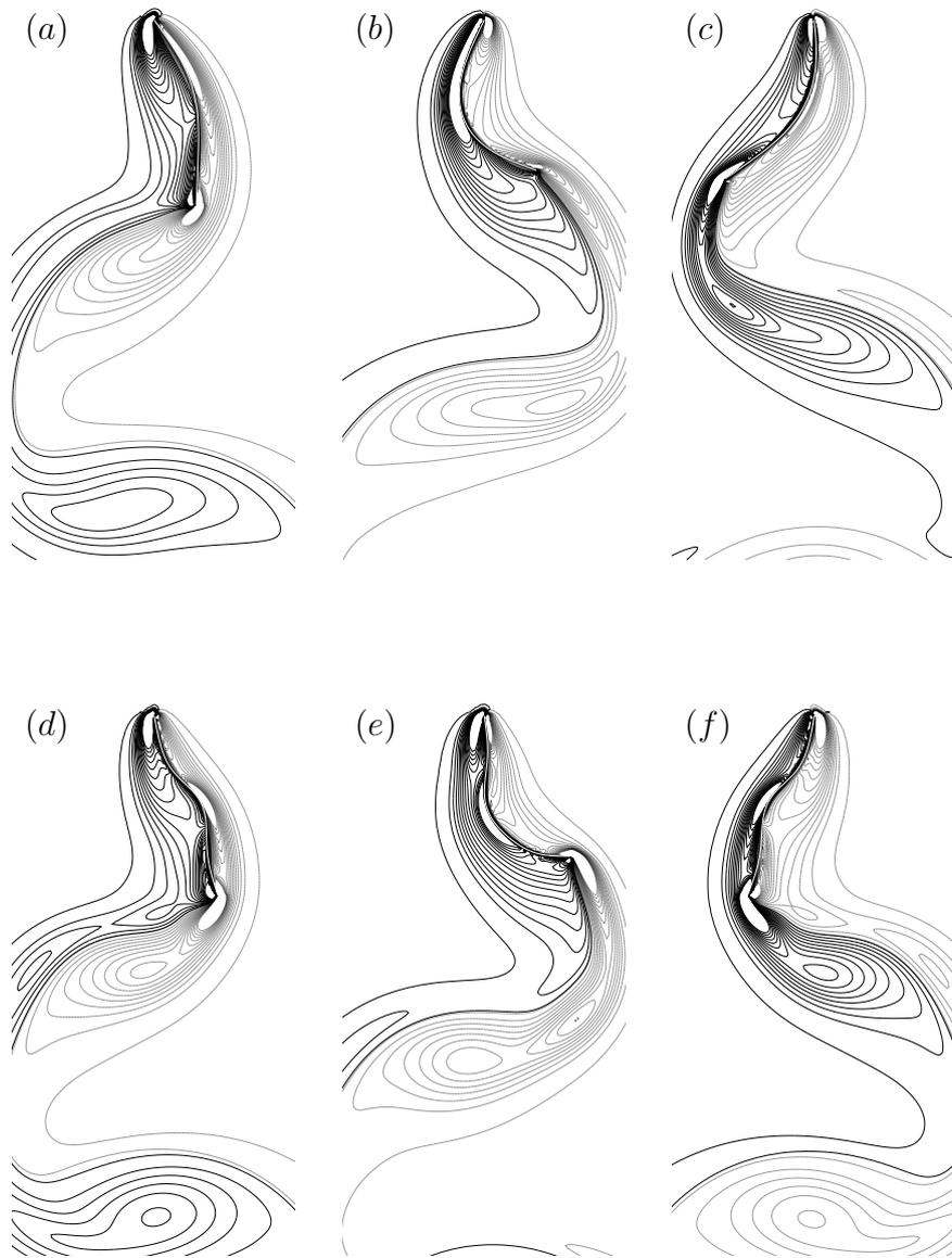
Figure 3.2.1: Vorticity iso-contours around impermeable flapping filament ( $Re = 200$ , positive vorticity in black, negative in gray) obtained with the code presented in Section 7.1.
