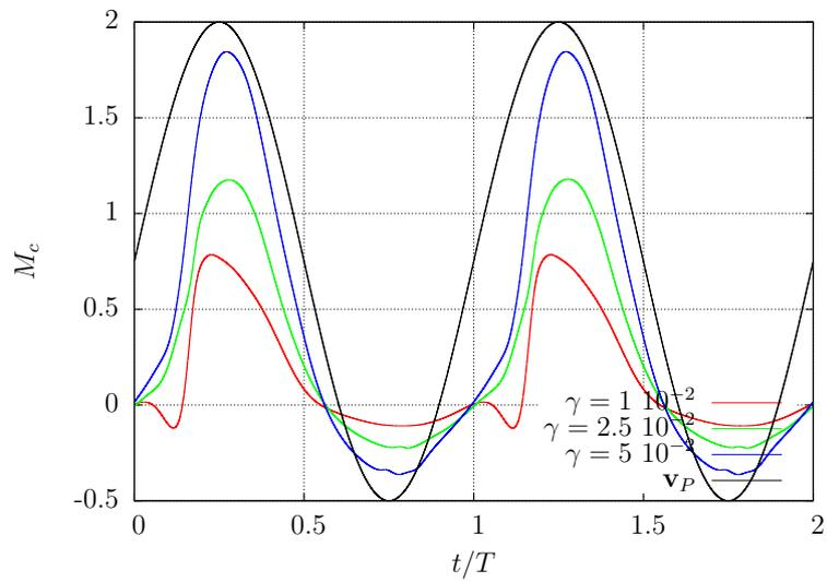
Figure 7.2.26: Time history of the moment acting at the attachment point of the filament for different bending stiffness and plate oscillation frequency  $\bar{f}$ . The velocity of the plate is in black.
