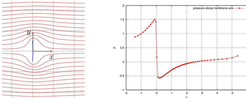
Figure 6.5.15: An inextensible membrane (left, solid line) simply supported at both ends is subject to a uniform flow from left (streamlines in dot lines) and (right) pressure profile along  $x$ . Notice the sudden pressure drop around membrane location ( $x \simeq 0$ ) within the space of two mesh grids.
