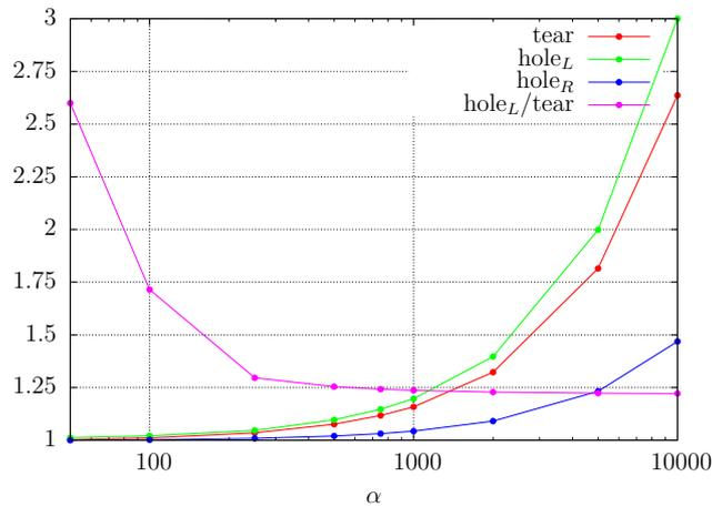
Figure 7.2.37: Tendency to detachment in the tear and hole configuration and ratio between them for  $L = 1$  and  $\theta = 33.56^\circ$ . As  $\alpha \rightarrow +\infty$  the ratio between the tear case and the hole left filament converges to 1.22, the ratio between the maximum torque for the respective cases.
