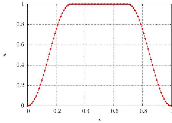
Figure 6.5.4: Regularized tangential velocity profiles along sliding wall for  $p = 0.4$ .
