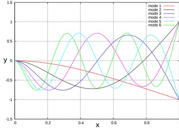
Figure 3.4.1: First natural modes of oscillations for the clamped beam normalized by the maximum amplitude.
