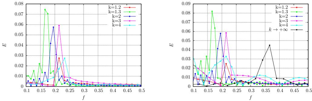
Figure 7.3.6: Frequency spectra for the leading (left) and trailing (right) edge. In the right graphics the spectrum for the case  $k \rightarrow +\infty$  is also shown.
