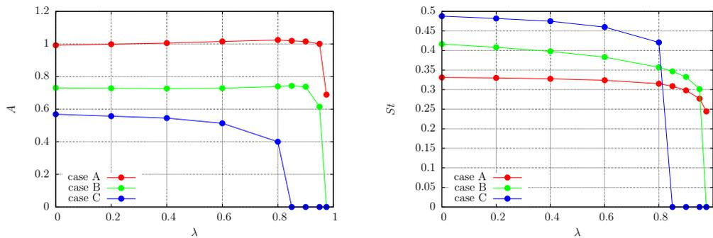
Figure 7.1.7: Oscillation amplitude and frequency as function of permeability. Each curve is drawn for different sets of parameters  $(\gamma, \rho)$ , see Figure 7.1.5.
