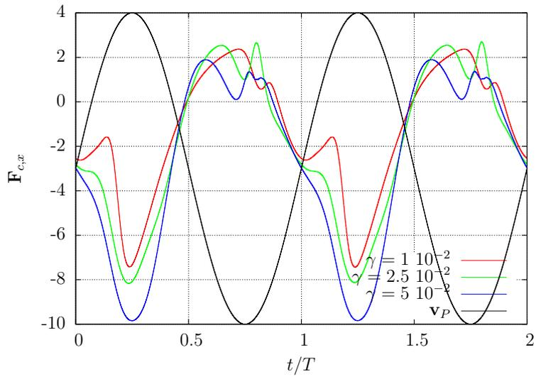
Figure 7.2.30: Time history of the x-force component acting at the attachment point of the filament for different bending stiffness and plate oscillation frequency  $0.25\bar{f}$ . The velocity of the plate is in black.
