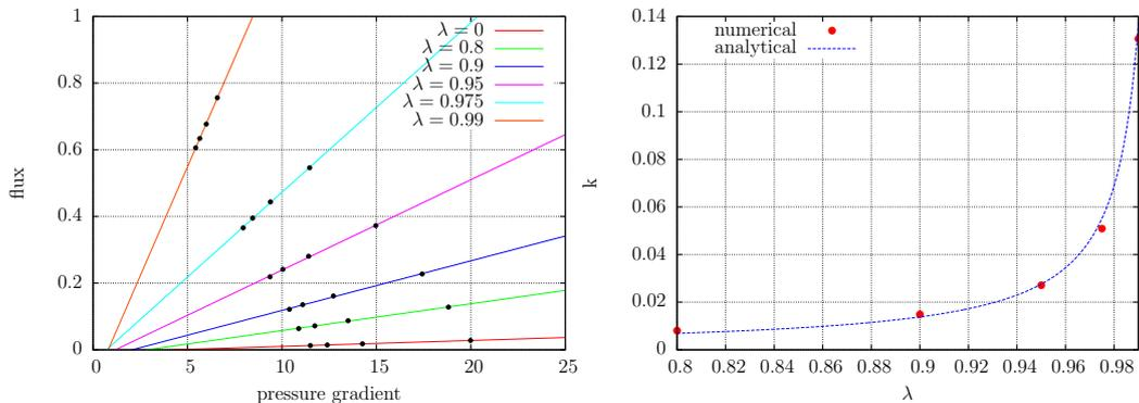
Figure 6.5.16: Linear regression of every set of simulations (dots) at different  $\lambda$  (left). Darcy’s  $k$  is the slope of each line and comparison between analytical prediction and numerical results of the  $k - \lambda$  mapping (right).
