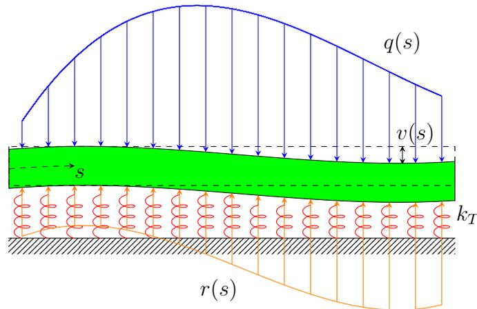
Figure 7.2.34: Foundation beam (in green) subject to an external load  $q(s)$  (in blue),  $s$  being the curvilinear abscissa, and supported by elastic spring of stiffness  $k_T$  (in red). The soil reaction  $r(s)$  (in orange) is proportional to the foundation displacement  $v(s)$ .
