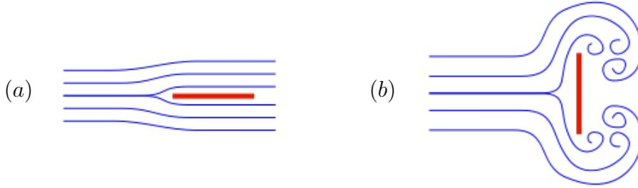
Figure 2.1.2: In the case of a flat plate aligned with the flow (a) the main part of the drag is due to friction, whereas in the case of plate perpendicular to the flow (b) the main part of the force is due to the pressure distribution around the plate.
