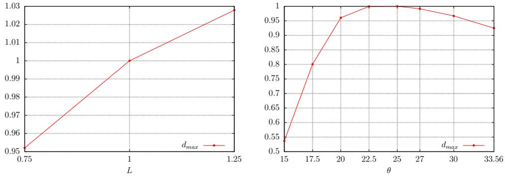
Figure 7.2.47: Maximum values of the tendency to detachment  $d$  for the tear case for different filament lengths  $L$  and  $\theta = 33.56^\circ$  (left), and for different  $\theta$  and  $L = 1$  (right).
