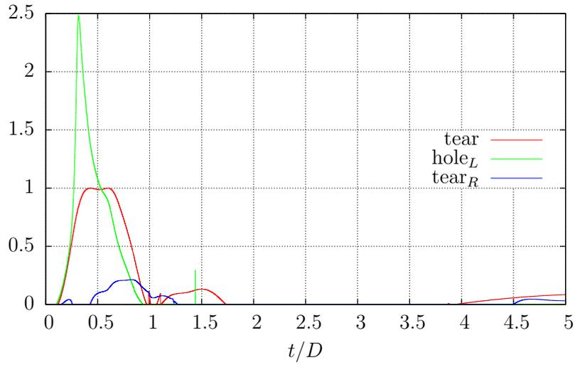
Figure 7.2.42: Tendency to detachment for the tear and hole case (right and left filaments) scaled with the maximum tendency to detachment in time for the tear configuration. Simulations for  $L = 0.75$  and  $\theta = 33.56^\circ$ .
