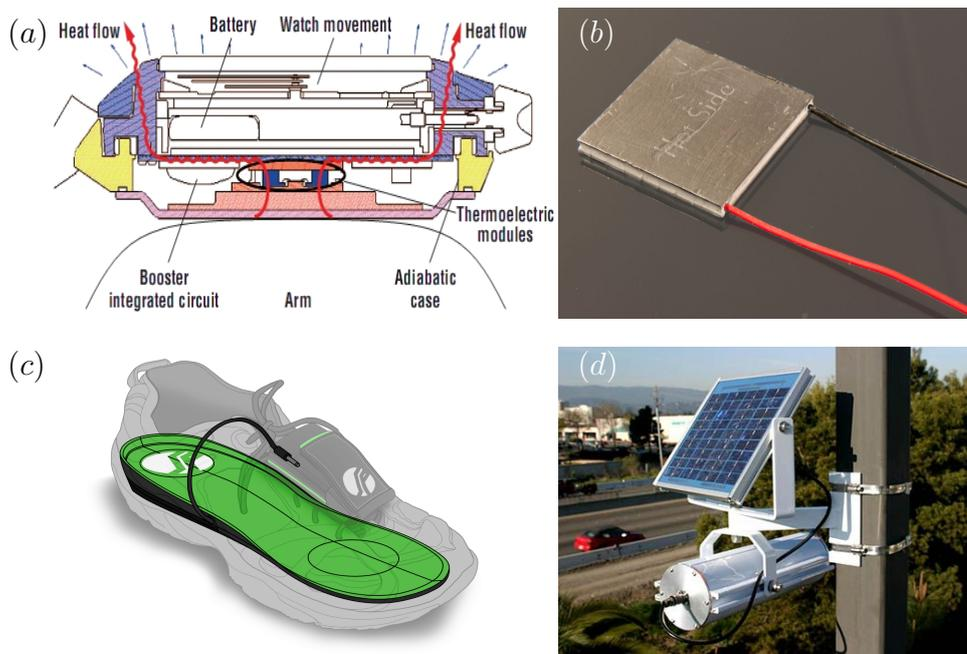
Figure 7.3.1: Energy harvesting applications: schematics of the Seiko Thermic wristwatch using the Peltier-Seebeck effect (a), thermoelectric (or TEG) generator generating electricity when a temperature difference is applied between the two faces of the module (b), SolePower EnSole producing energy for storage in the battery inside the holster (c) and a solar panel powering the remote sensor located at a several-meter high location (d).
