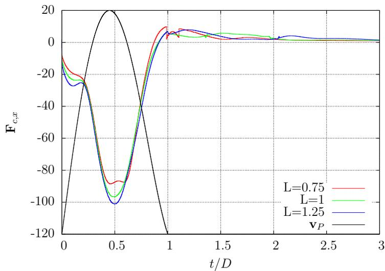
Figure 7.2.6: Time history of the x-force component acting at the attachment point of the filament for different filament lengths. The velocity of the plate is in black.
