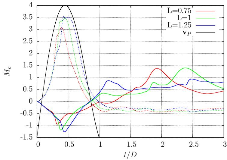
Figure 7.2.16: Time history of the moment acting at the attachment point of the right (line) and left (dots) filament for different filament lengths. The velocity of the plate is in black.
