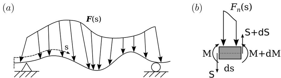
Figure 3.3.1: 1-d beam with a distributed load  $\mathbf{F}(s)$  along its axis (a) and an infinitesimal element of the beam with its internal strains  $S$  and torque  $M$ (b).
