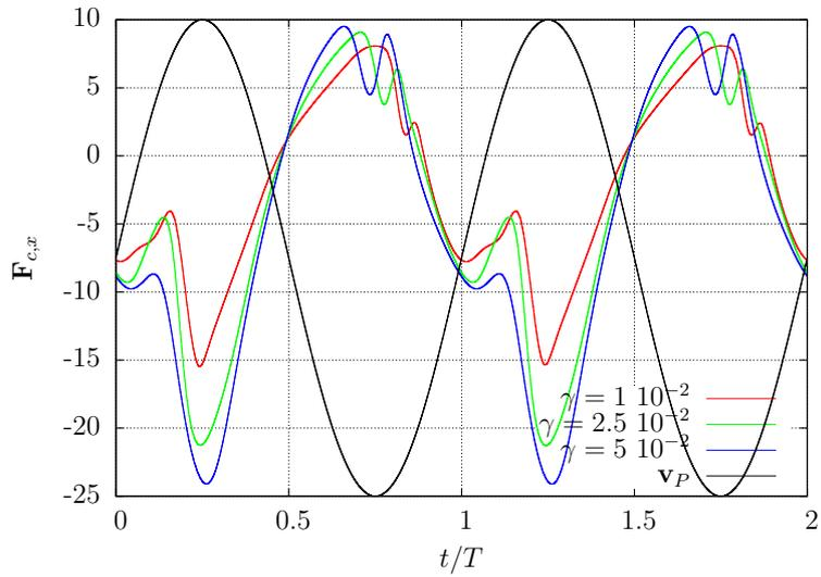
Figure 7.2.27: Time history of the x-force component acting at the attachment point of the filament for different bending stiffness and plate oscillation frequency  $0.5\bar{f}$ . The velocity of the plate is in black.
