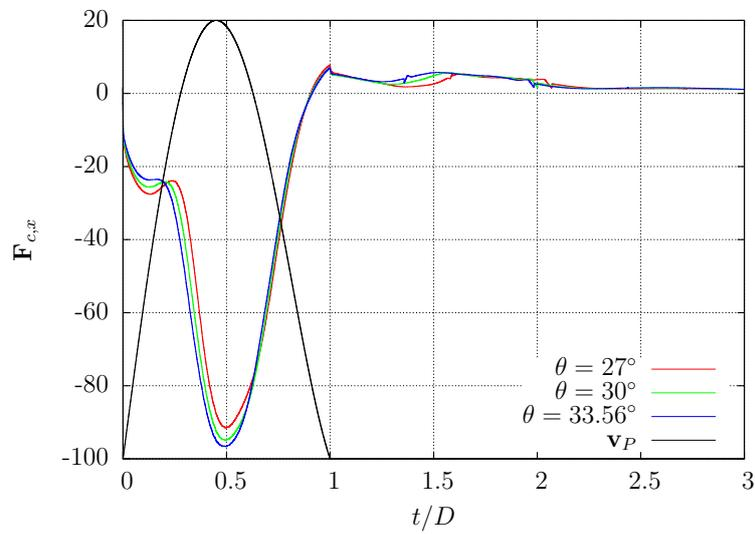
Figure 7.2.9: Time history of the x-force component acting at the attachment point of the filament for different filament angles. The velocity of the plate is in black.
