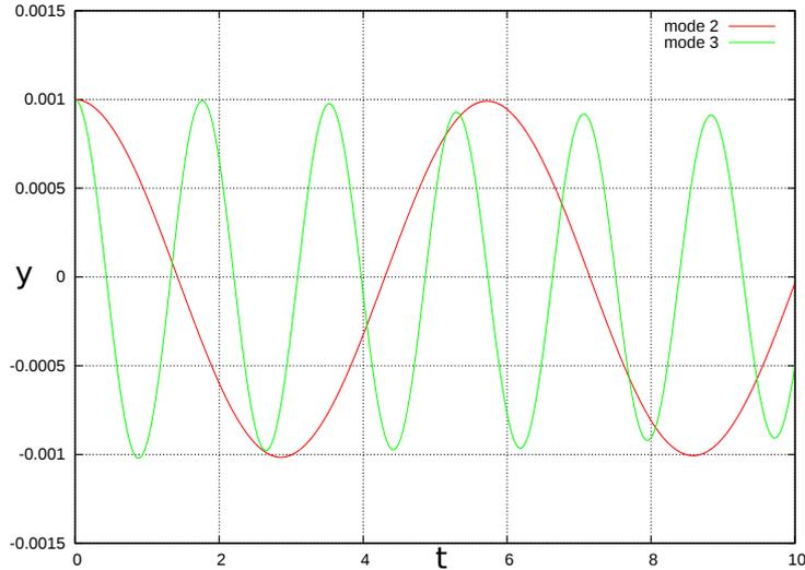
Figure 6.5.12: Time trace of displacement at the hinged beam's free end.
