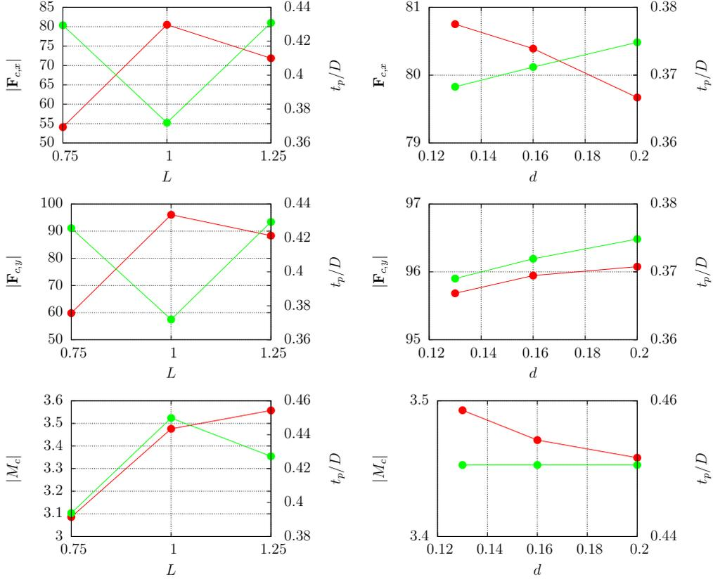
Figure 7.2.21: Peak values (in red) of force component  $|\mathbf{F}_{c,x}|$  (first row),  $|\mathbf{F}_{c,y}|$  (second row), and moment  $|M_c|$  and corresponding time (in green) for the left filament in the “hole” case. The left column shows the values for different filament length  $L$ , while in the right column the inter-tip distance  $d$  varies.
