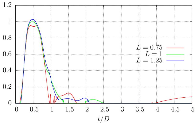
Figure 7.2.45: Tendency to detachment for the tear case with different lengths and  $\theta = 33.56^\circ$ . Results have been scaled with the maximum tendency to detachment in time for  $L = 1$ .
