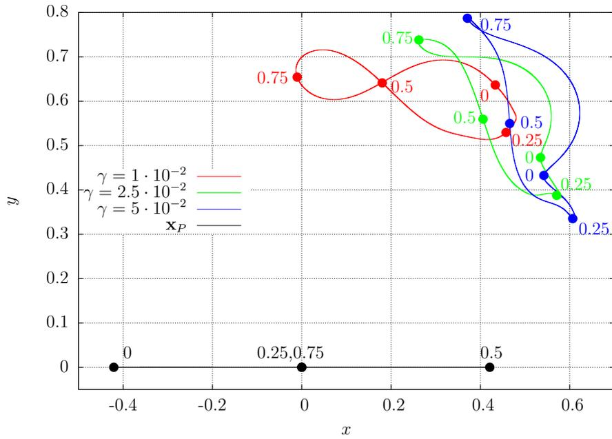
Figure 7.2.23: Trajectory of the filament tip for different bending stiffness and of the plate (black). The colored dots indicate the simulation time (as indicated in Figure 7.2.22 and 7.2.24-7.2.26).
