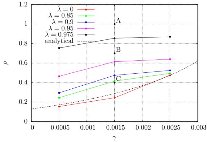
Figure 7.1.5: Neutral curve on the plane  $(\gamma, \rho)$  for  $Re = 200$  and  $\lambda = 0$ . The analytical curve for  $\lambda = 0$  is taken from [70], whereas dotted lines represent neutral curves for different permeabilities.
