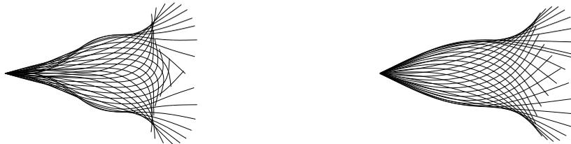
Figure 7.1.3: Snapshots of impermeable filament during one flapping cycle for case D (left) and E (right) depicted on Figure 7.1.2. While a unique concavity characterizes the behavior of the right filament, an inflection point is clearly identifiable in the left oscillations.
