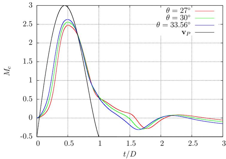
Figure 7.2.11: Time history of the moment acting at the attachment point of the filament for different filament angles. The velocity of the plate is in black.
