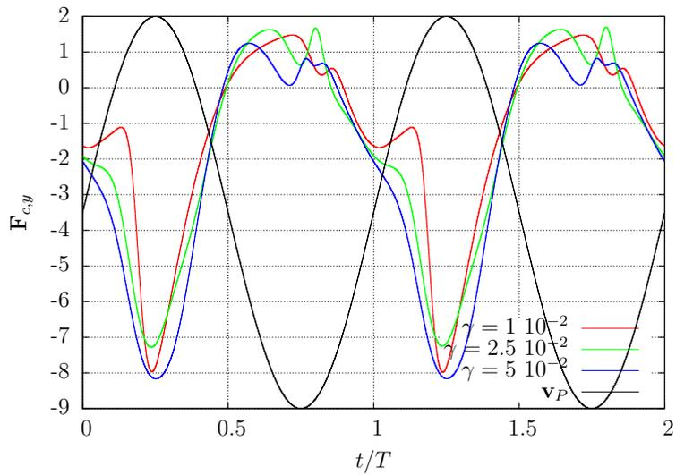
Figure 7.2.31: Time history of the y-force component acting at the attachment point of the filament for different bending stiffness and plate oscillation frequency  $0.25\bar{f}$ . The velocity of the plate is in black.
