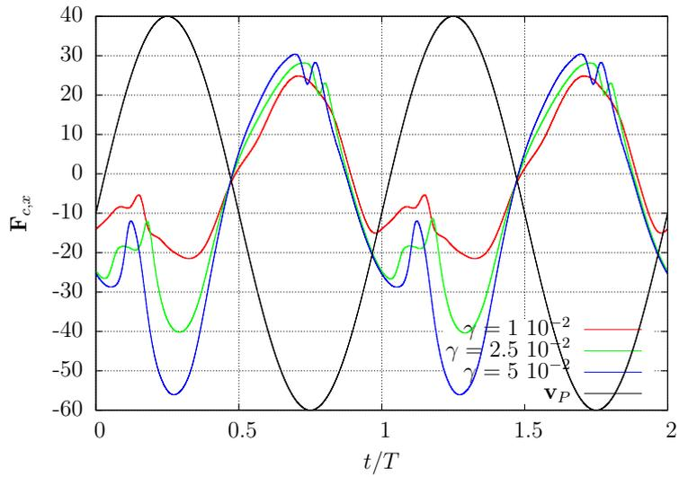
Figure 7.2.24: Time history of the x-force component acting at the attachment point of the filament for different bending stiffness and plate oscillation frequency  $\bar{f}$ . The velocity of the plate is in black.
