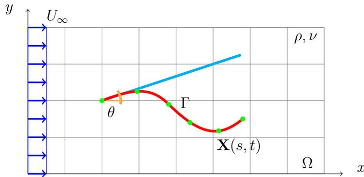
Figure 7.1.1: Filament  $\Gamma$  (in red) described by a set of Lagrangian points  $\mathbf{X}(s, t)$  (in green). Initial configuration (in cyan) of the filament is a straight line with a certain angle of attack  $\theta$ .
