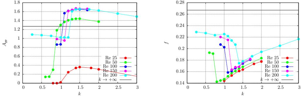
Figure 7.3.8: Flapping peak-to-peak amplitude (left) and frequency (right) of the trailing edge for different Reynolds numbers.
