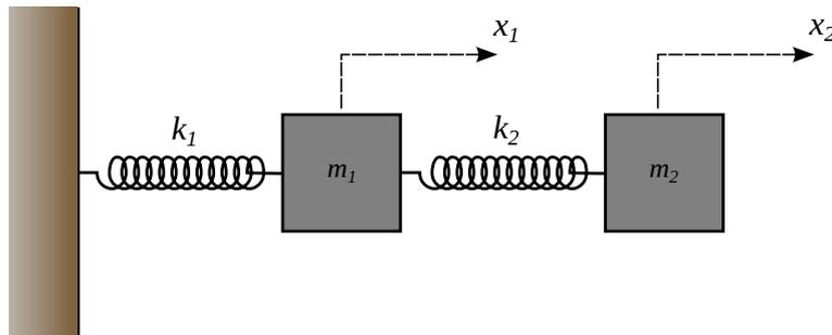
Figure 3.1.1: Dynamical system made up of two masses  $m_1$  and  $m_2$  linked by springs of different elastic constant  $k_1$  and  $k_2$  to an external wall.
