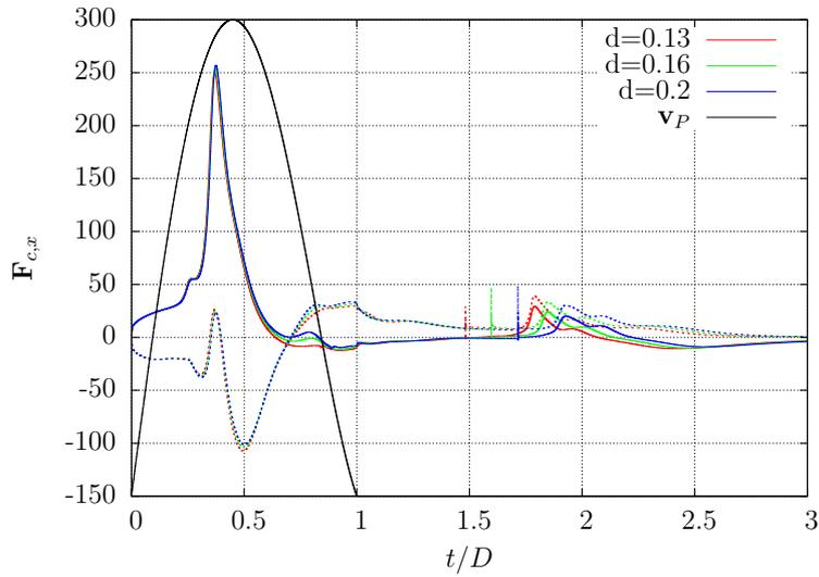
Figure 7.2.17: Time history of the x-force component acting at the attachment point of the right (line) and left (dots) filament for different inter-tip distances. The velocity of the plate is in black.
