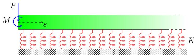
Figure 7.2.35: Semi-infinite foundation beam (in green) subject to a punctual force  $F$  and torque  $M$  at the finite end.
