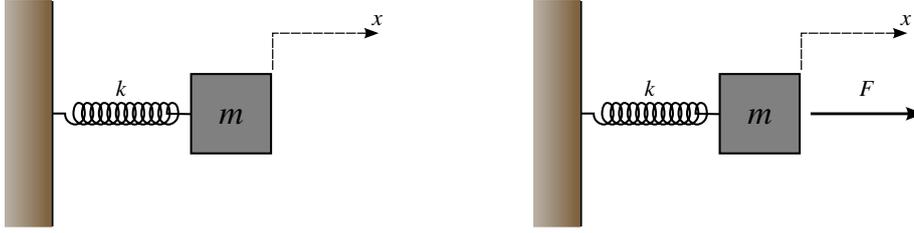
Figure 3.1.2: Unforced (left) and forced (right) spring-mass system.
