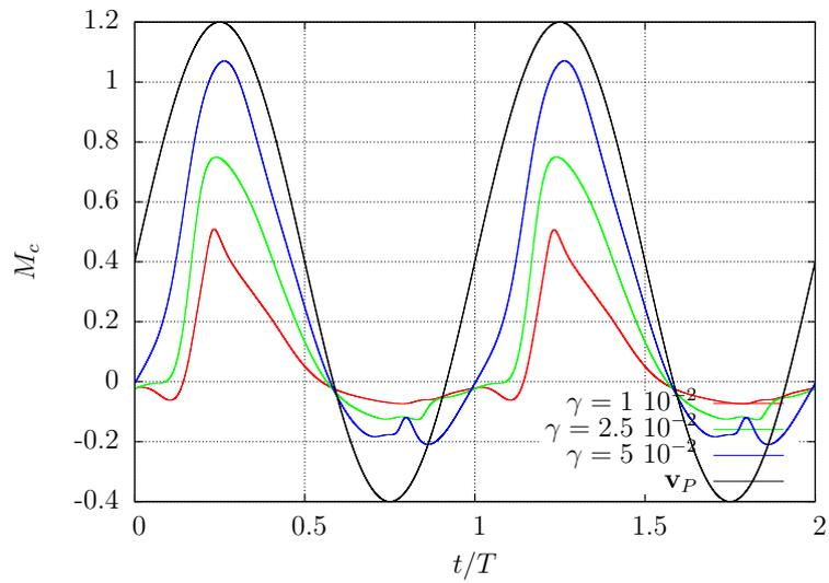
Figure 7.2.29: Time history of the moment acting at the attachment point of the filament for different bending stiffness and plate oscillation frequency  $0.5\bar{f}$ . The velocity of the plate is in black.
