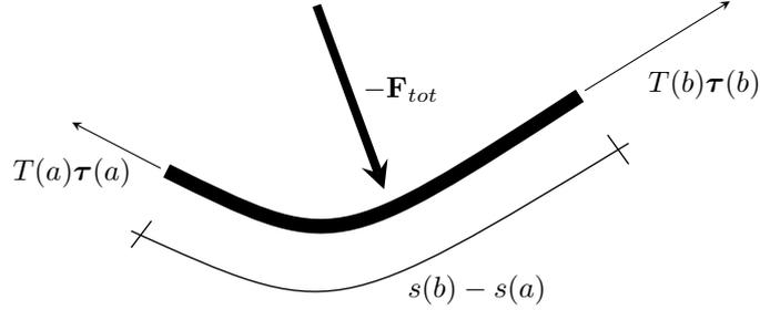
Figure 5.2.1: Equilibrium condition on a small element of membrane.
