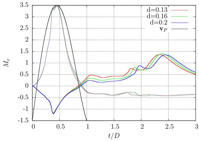
Figure 7.2.19: Time history of the moment acting at the attachment point of the right (line) and left (dots) filament for different inter-tip distances. The velocity of the plate is in black.
