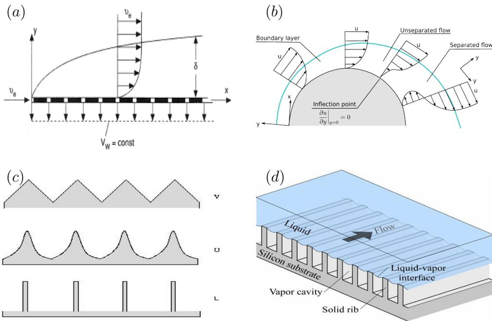
Figure 2.2.1: Different passive flow control techniques: suction surfaces for delaying transition (a), surface shaping for delaying boundary layer detachment (b), different riblet pattern (c) and super-hydrophobic surface (d).
