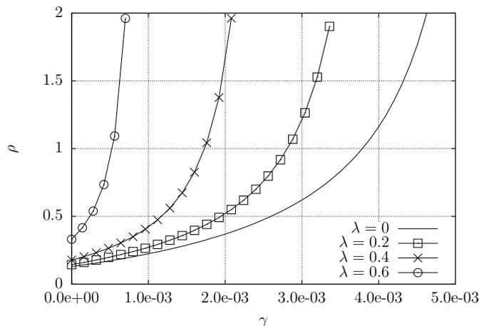
Figure 7.1.11: Neutral curves on the plane  $(\gamma, \rho)$  for  $Re = 200$  and different values of the permeability coefficient  $\lambda$ .
