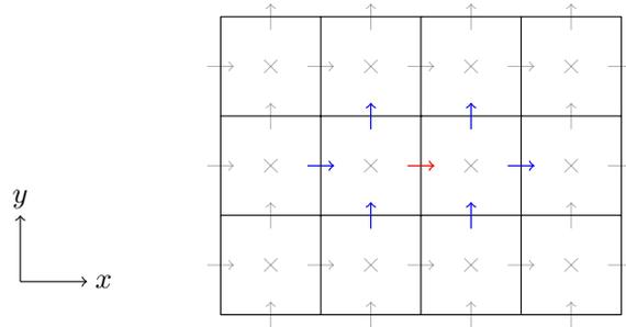
Figure 6.1.3: Non-linear operator stencil (in blue) for an  $x$ -component velocity node (in red).
