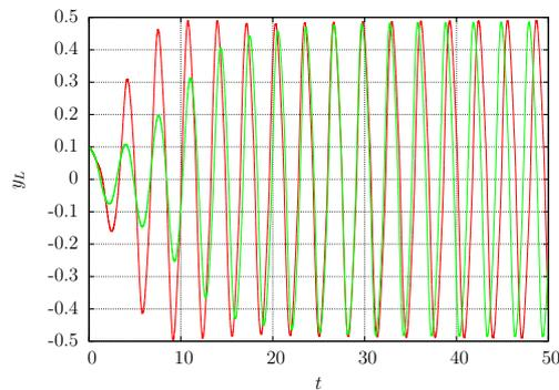
Figure 7.1.4: Y-coordinate of impermeable filament trailing edge for case D (red) and E (green) depicted on Figure 7.1.2.
