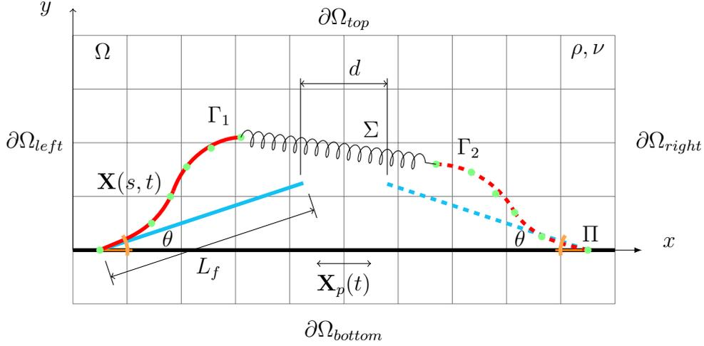
Figure 7.2.4: Filament  $\Gamma_1$  (in red, initial condition in cyan) is clamped to an underlying plate  $\Pi$  with a certain angle  $\theta$  and is described by a set of Lagrangian points  $\mathbf{X}(s, t)$  (in green). Plate  $\Pi$  is animated with a prescribed motion  $\mathbf{X}_p(t)$ . In the “hole” case filament  $\Gamma_2$  is also considered, bounded by spring  $\Sigma$  to  $\Gamma_1$  with initial distance  $d$  (always kept constant).
