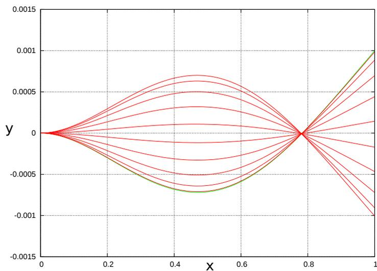
Figure 6.5.11: Beam snapshots during one oscillation. Initial condition (in green) is such that only the second oscillation mode is excited.
