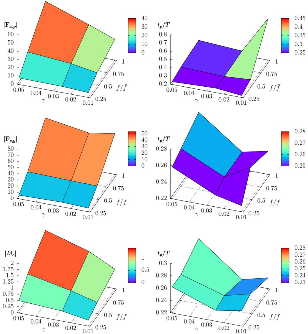
Figure 7.2.33: Surface plots of the peak values (right column) of force components  $|\mathbf{F}_{c,x}|$  (first row),  $|\mathbf{F}_{c,y}|$  (second row) and moment  $|M_c|$  (third row) and their corresponding time  $t_p/T$  (left column) for the “periodic” case as a function of the bending stiffness  $\gamma$  and of the plate oscillation frequency  $f/\bar{f}$ .
