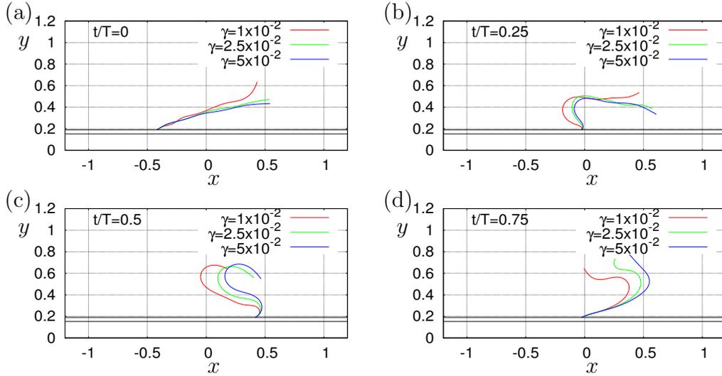
Figure 7.2.22: Dynamics of the single clamped filament during the oscillating plate motion at different times. The trajectory of the filament tip is shown in Figure 7.2.23.
