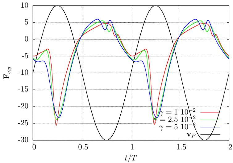
Figure 7.2.28: Time history of the y-force component acting at the attachment point of the filament for different bending stiffness and plate oscillation frequency  $0.5\bar{f}$ . The velocity of the plate is in black.
