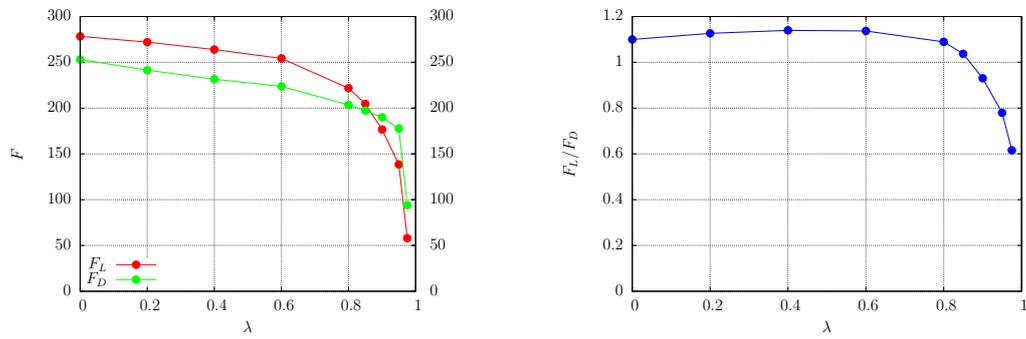
Figure 7.1.8: Lift and drag forces (left) aerodynamic efficiency (right) for case A (Figure 7.1.5), all as a function of the permeability.
