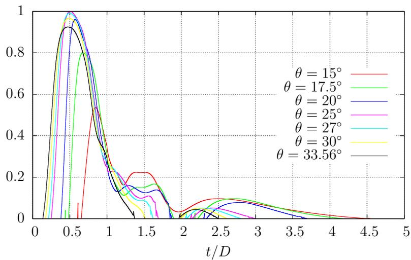
Figure 7.2.46: Tendency to detachment for the tear case with different clamping angles and  $L = 1$ . Results have been scaled with the maximum tendency to detachment in time for  $\theta = 25^\circ$ .
