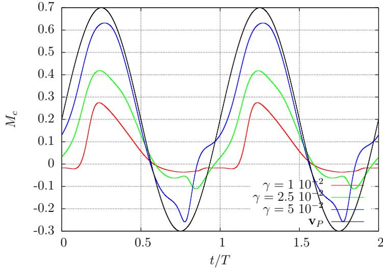
Figure 7.2.32: Time history of the moment acting at the attachment point of the filament for different bending stiffness and plate oscillation frequency  $0.25\bar{f}$ . The velocity of the plate is in black.
