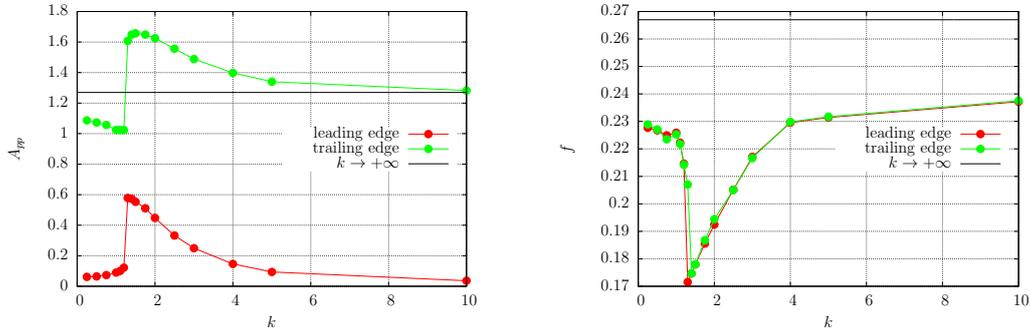
Figure 7.3.5: Flapping peak-to-peak amplitude (left) and frequency (right) of the leading and trailing edge once a stable oscillation state is reached. The solid line represents the peak-to-peak amplitude and flapping frequency of the hinged filament, i.e.  $k \rightarrow +\infty$
