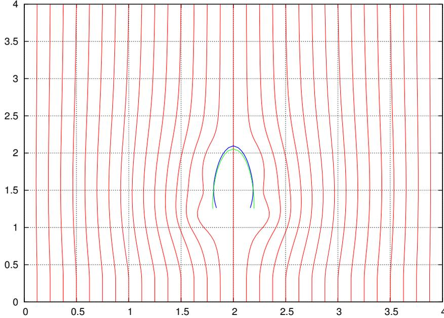
Figure 6.5.6: Streamlines (in red) around the opening parachute (in blue). The initial position of the parachute is shown in green.
