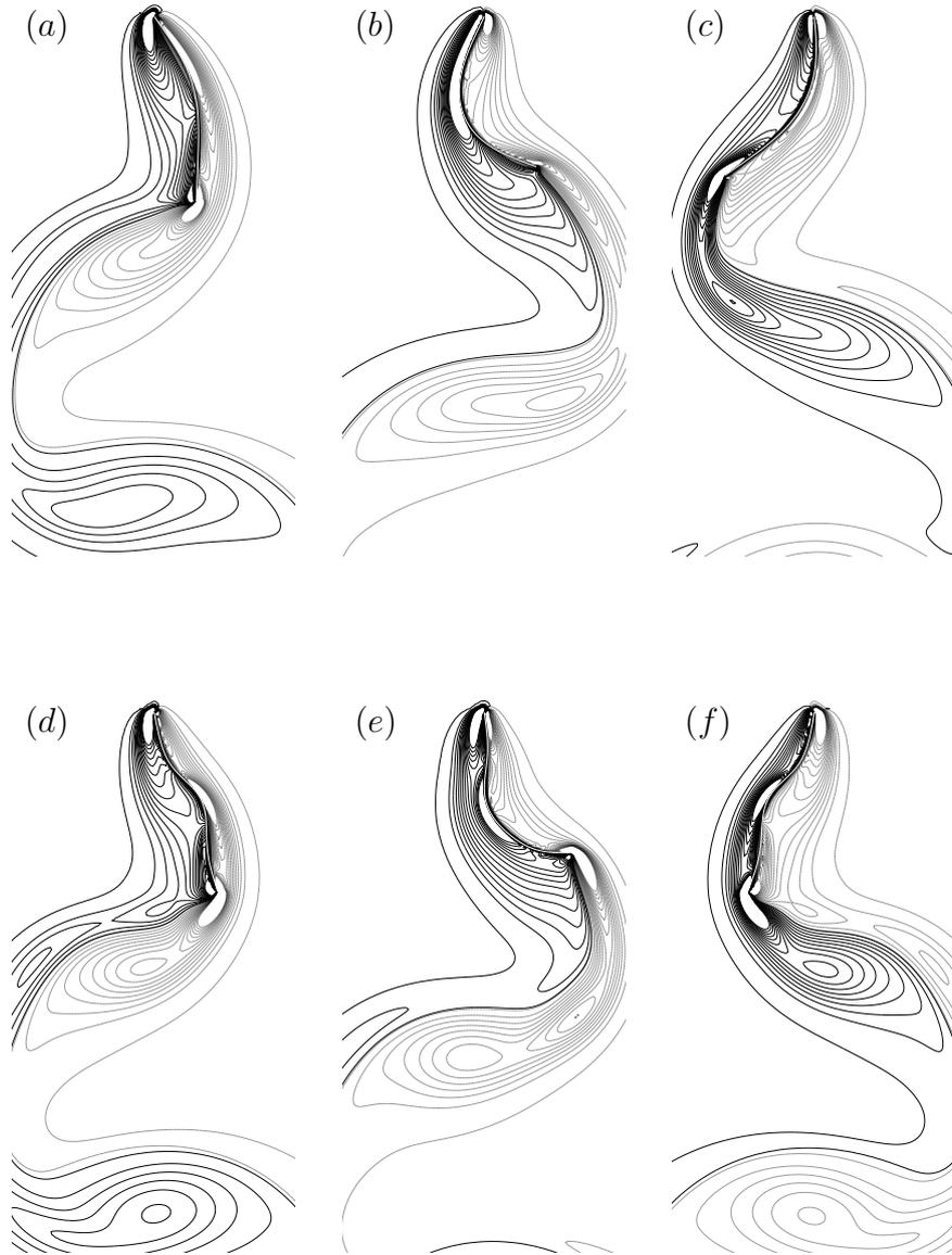
Figure 7.1.10: Vorticity iso-contours ( $[-15 : 15]$ ) around impermeable flapping filament ( $Re = 200$ , positive vorticity in black, negative in gray). With reference to Figure 7.1.2, snapshots  $(a, b, c)$  refer to case D ( $\rho = 1, \gamma = 2,5 \cdot 10^{-3}$ ) whereas  $(d, e, f)$  refer to case E ( $\rho = 1, \gamma = 15 \cdot 10^{-3}$ ).
