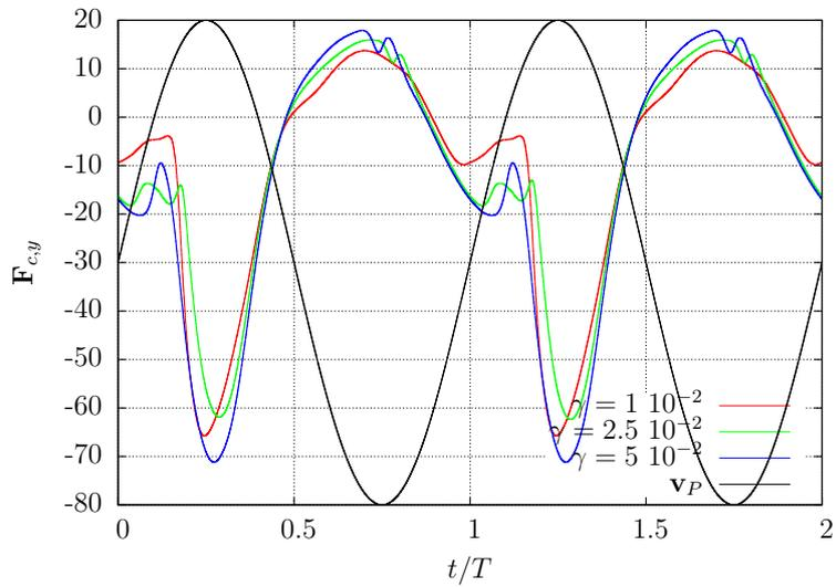
Figure 7.2.25: Time history of the y-force component acting at the attachment point of the filament for different bending stiffness and plate oscillation frequency  $\bar{f}$ . The velocity of the plate is in black.
