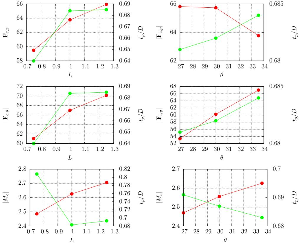
Figure 7.2.12: Peak values of force  $|\mathbf{F}_c|$  and moment  $|M_c|$  (in red) and corresponding time (in green) for the “tear” case. The left column shows the values for different filament length  $L$ , while in the right column the clamping angle  $\theta$  varies.
