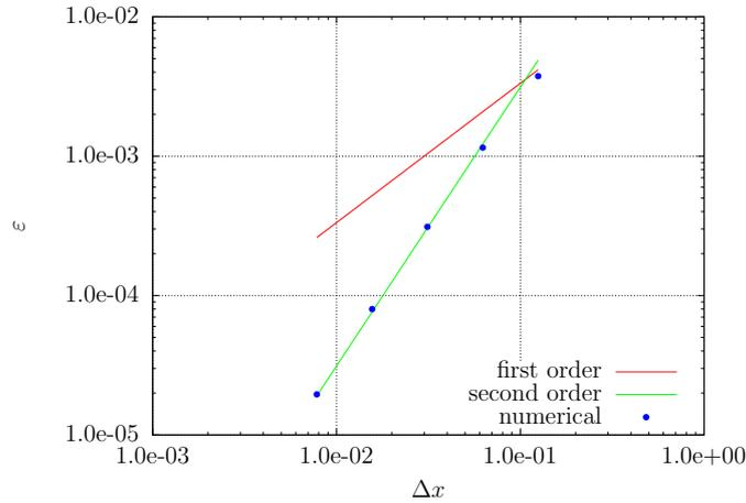
Figure 6.5.2: Spatial convergence rate of the numerical code (dots) compared with the theoretical first- and second-order error curves.
