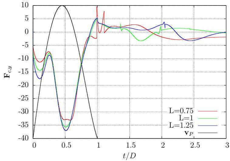
Figure 7.2.7: Time history of the y-force component acting at the attachment point of the filament for different filament lengths. The velocity of the plate is in black.
