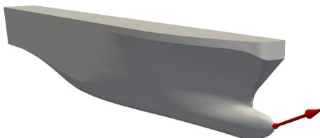
Figure 13.1: *Example of shape morpher inputs: control point (bulb's nose) and displacement ( $x = 0.4[m]$  and  $z = 0.2[m]$ ).*
