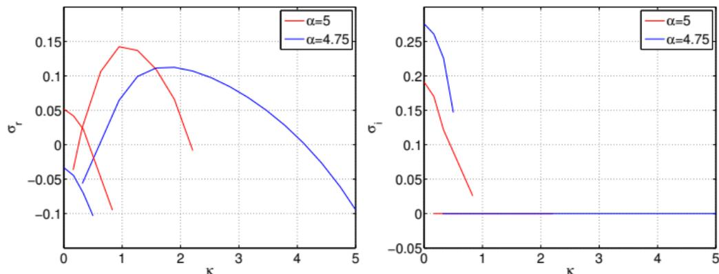
Growth rate  $\sigma_r$  (left) and Strouhal number  $St = \sigma_i/(2\pi)$  (right) for  $Re = 100$  as a function of the rotation rate and spanwise wave number.
