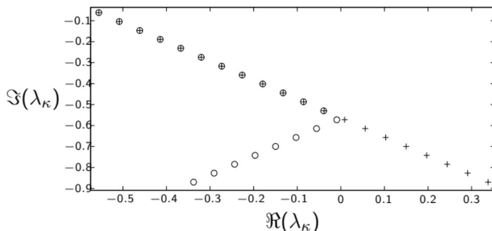
The eigenvalues of (+) the discretized open-loop system, and (o) the closed-loop system  $A + BK$  after minimal-energy control is applied.
