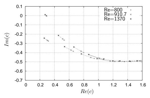
Temporal eigen value spectrum of the Blasius boundary layer for three values of Re, with  $\alpha=0.086$ . At Re=910.7 Im(c)=0 for the least stable eigen value. The "old" continuous spectrum: Re(c)=1. Bottom: including trajectories of the discrete eigen values
