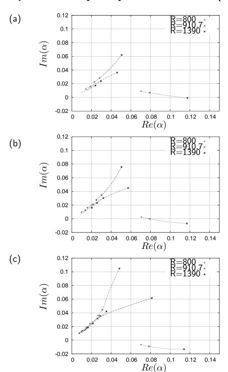
Spatial eigen value spectrum,  $\alpha$ , three values of the Reynolds number, given  $F=25.10^{-6}$ . The pressure gradient in the mean flow is given by the Hartree parameter (a)  $\beta_H=0.1$ , (b)  $\beta_H=0$ , (c)  $\beta_H=-0.1$ .
