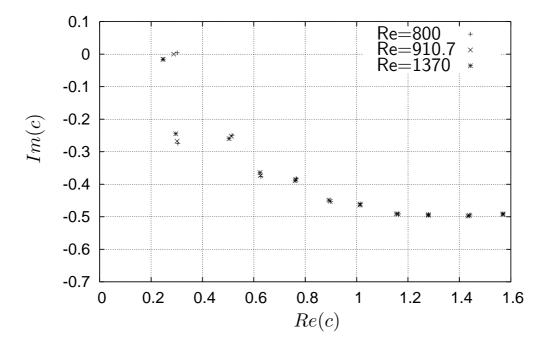
Temporal eigen value spectrum for three values of Re, keeping the value of  $\alpha Re$  constant. At Re=910.7,  $\alpha$  is chosen such that Im(c)=0 for the least stable eigen value.
