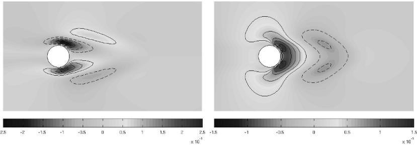
**Fig. 2**  $K$  for  $l \rightarrow \infty$  (Minimum energy control),  $Re = 55$ ; (left)  $K_u$ , (right)  $K_v$ . Solid contours indicate positive values and dashed negative values.
