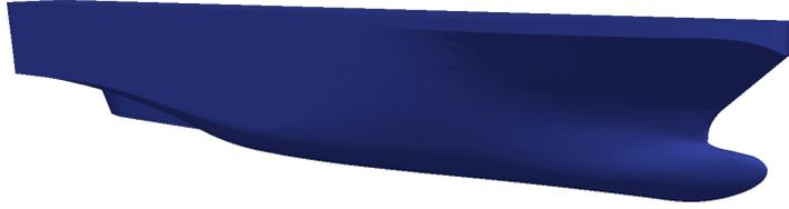
Using *CAMILO* shape morpher, bulb's nose is displaced forward and backward. Seven nose displacements are performed:
