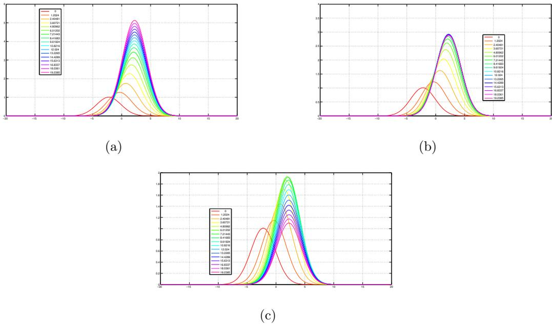
Figure 3: Different evolution of the initial perturbation in a (a) unstable ( $\sigma_0 = 0.5$ ), (b) neutral ( $\sigma_0 = 0.47$ ) and (c) stable ( $\sigma_0 = 0.42$ ) sets of parameters. Note in the last figure the transient growth before the decaying of the perturbation.
