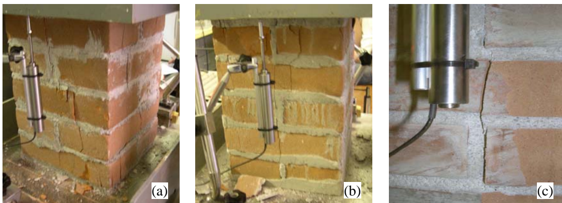
Figure 8: Cracking of masonry prisms at 80% of the peak load: a) and b) lateral views; c) detail.
