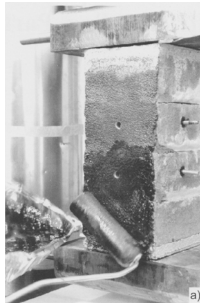
Fig. 1 a - The surface is prepared with a controlled mixture of cement and fillers.
