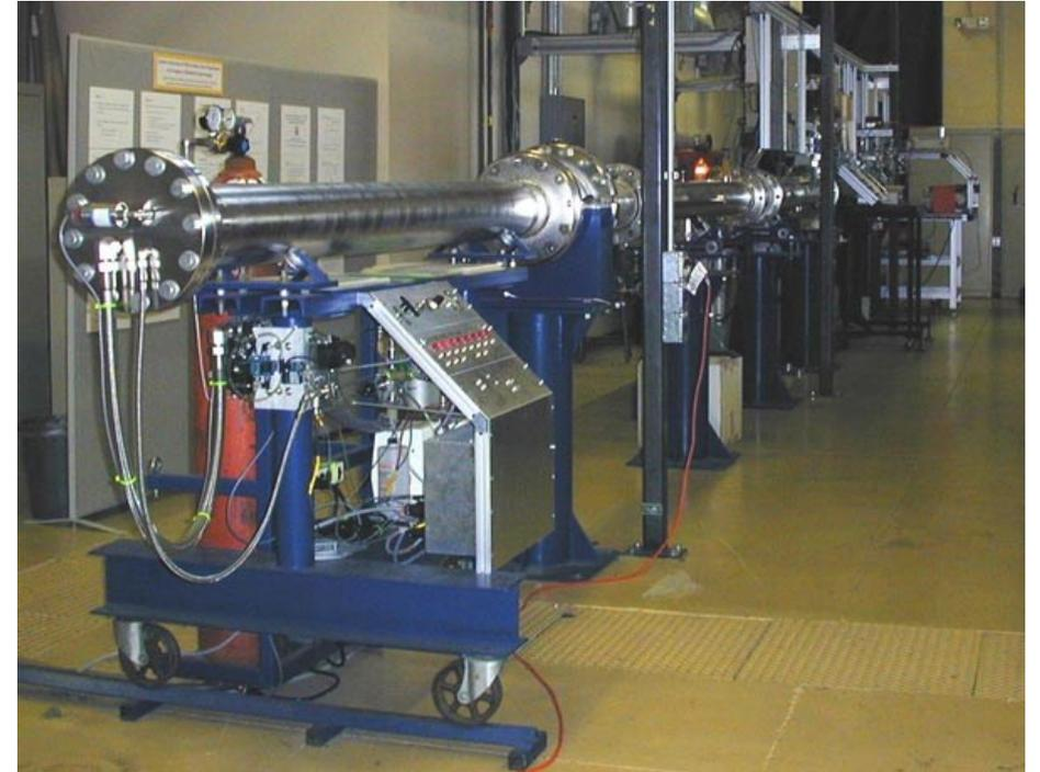
**Shock tube. The driver section, including vacuum pumps, controls, and helium driver gas.**
