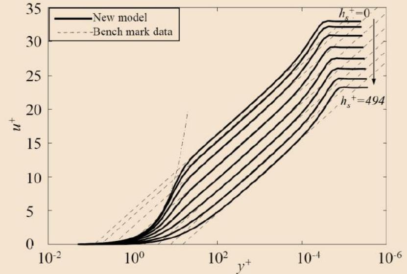
Plot of roughness mean velocity profiles [2].
