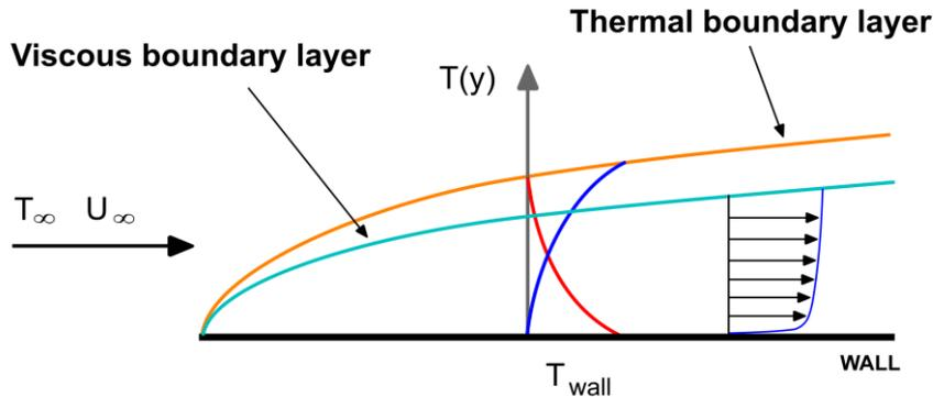
Thermal boundary layer vs. Viscous boundary layer
