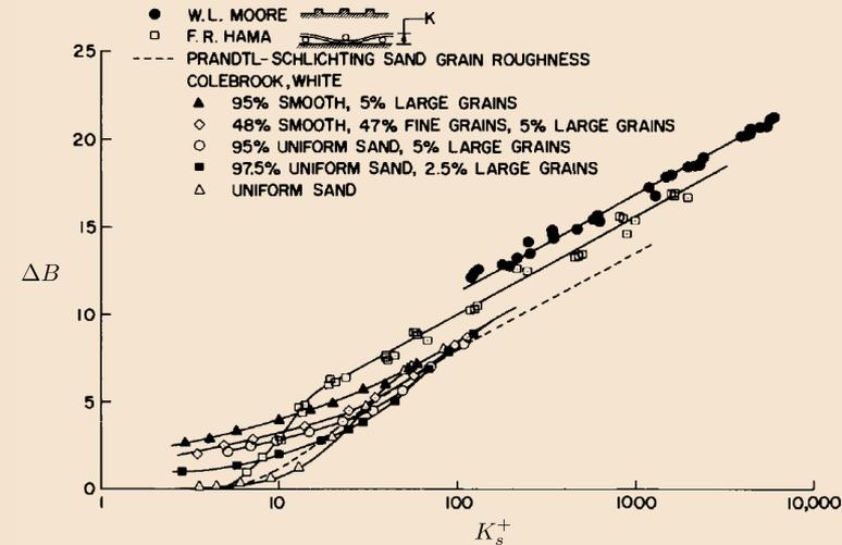
Effect of wall roughness on the roughness correction factor and universal velocity profiles [3].
