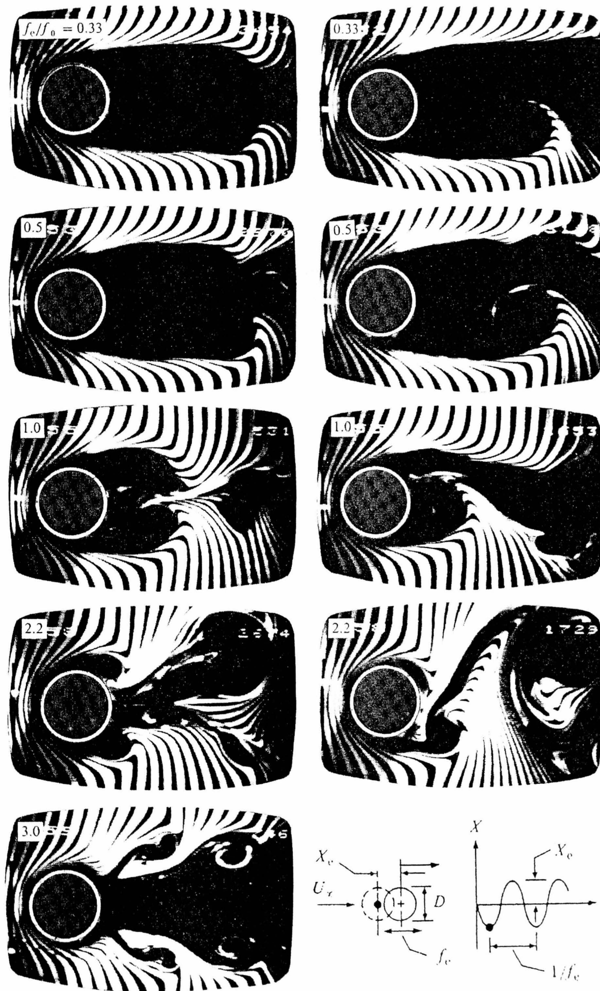
Figure 2.35 Comparison of asymmetrical and symmetrical shedding modes for a circular cylinder. All images taken at the moment corresponding to maximum upstream cylinder displacement, from Ongoren and Rockwell (1988b).
