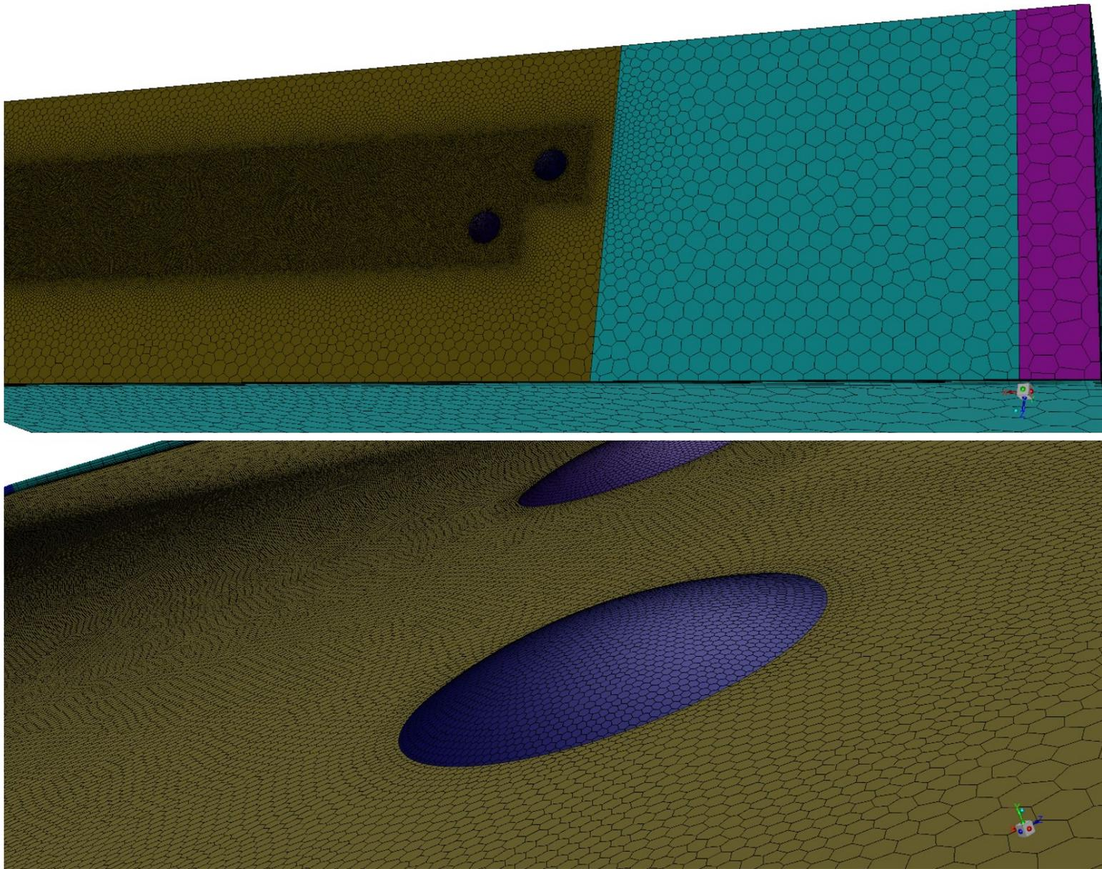
The mesh is first generated on surfaces and then the whole volume is filled using polyhedrons and hexahedrons
