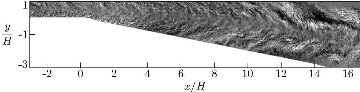
Figure 20: Instantaneous spanwise velocity from LES of the 3D diffuser of Kolade (2010) at  $z/H \approx 1.67$ . Contours from  $-0.2U_b$  to  $0.2U_b$  [51].
