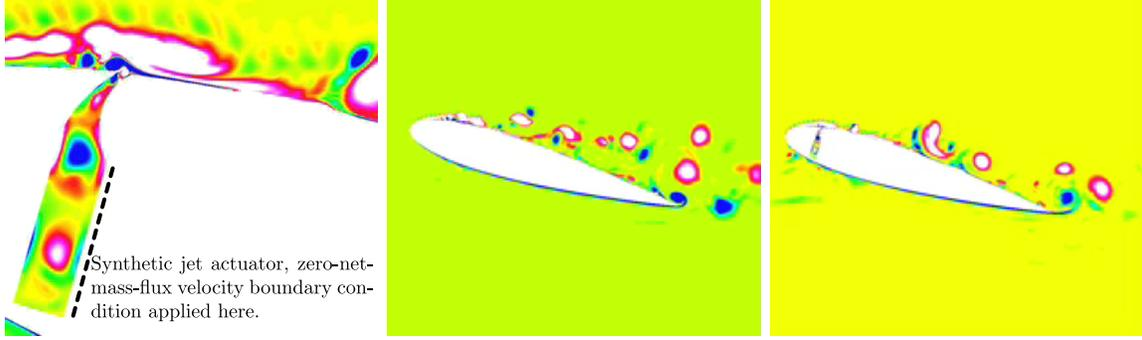
Figure 14: Instantaneous spanwise vorticity contours of flow over a NACA 0015 airfoil with synthetic jet actuation (left) without control (middle) and with control (right) [56].
