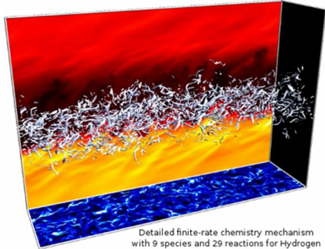
Figure 10: Supersonic temporal mixing layer Q-criterion isosurfaces. Density contours in background; centerline strain-rate projected below.
