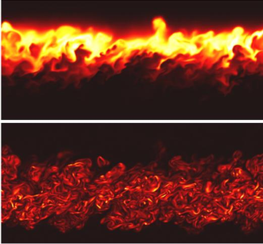
Figure 9: Instantaneous OH mass fraction (top) and vorticity magnitude (bottom) in a plane normal to span.
