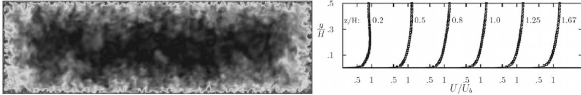
Figure 19: Left: instantaneous streamwise velocity in the  $yz$ -plane in a rectangular duct with cross-section  $3.33H \times H$ ; contour levels from 0 to  $1.4U_b$  [51]. Right: mean streamwise velocity profiles at different spanwise locations for the explicitly filtered LES (solid lines) and experimental measurements of Kolade (2010) (symbols).
