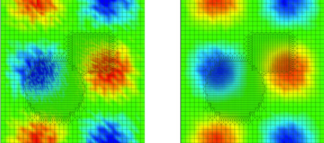
Figure 13: A sinusoidal function with superimposed random noise (20% amplitude) on an unstructured grid with local grid refinement: unfiltered (left) and filtered (right) [51].
