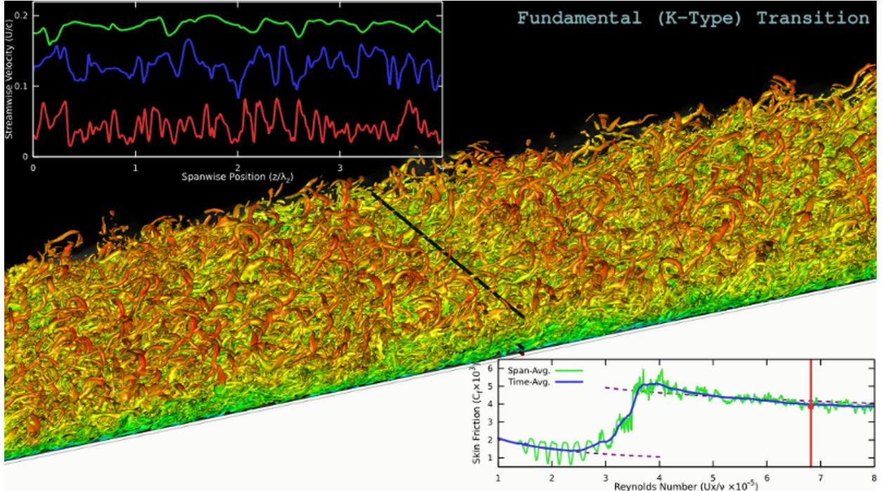
Figure 3b: See figure 3a for caption. This figure shows Reynolds number  $R_\theta \approx 1200$  flow over a flat plate boundary layer. Note how the boundary layer thickens and length scales become larger [20, 21]. Simulations of H/K-type transition performed on Intrepid at the Argonne Leadership Computing Facility (ALCF) and with dedicated time on the LLNL BGL machine for improved statistical sampling.
