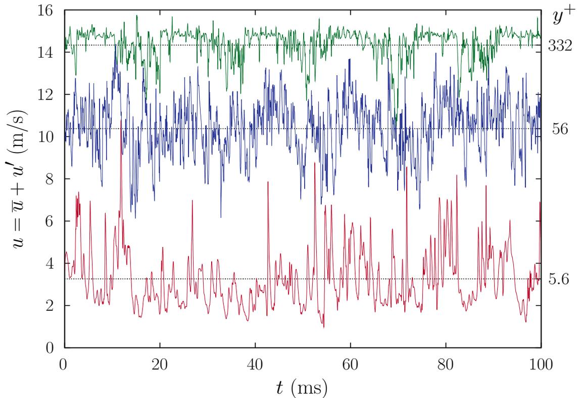
Figure 4a: Instantaneous streamwise velocities at three different heights from the wall at Reynolds number  $Re_\theta = 900$  from the boundary-layer simulation of [23]. Variables made dimensional assuming air flowing with free-stream velocity  $U_\infty = 15$  m/s along a wall, which corresponds to the velocity and time scales seen in the thin boundary layer on automobiles that is only a few millimeters thick.
