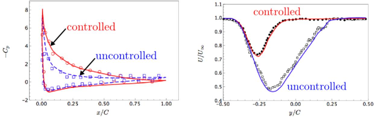
Figure 15: Validation of simulation (lines) against experimental data (symbols) without control (blue) and with control (red) with airfoil surface pressure coefficient (left) and velocity wake at  $x/C = 1.2$  (right) [56].
