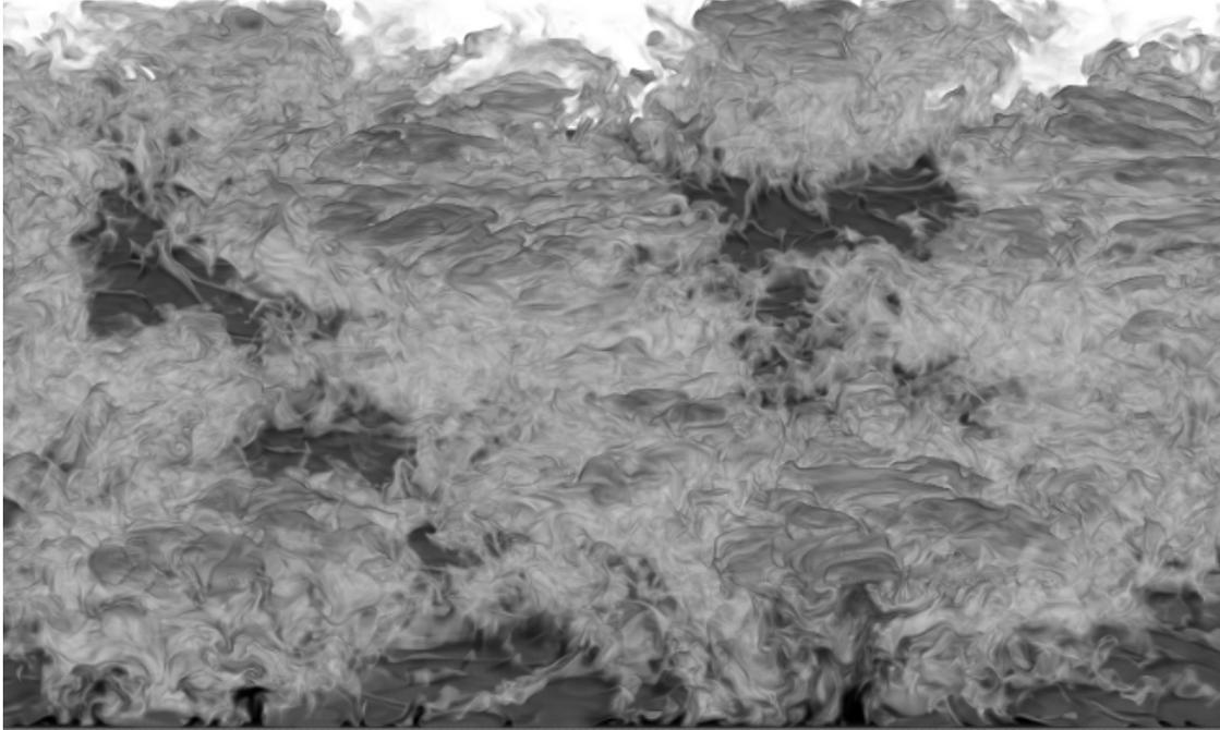
Figure 6: Isovolume rendering of thermal updrafts in air. The Reynolds number corresponds to the same flow conditions given in the text except the radiator is now a constant temperature floor heater. When the thermal plumes rise and come close to the cold wall, they spread out laterally creating flattened but corrugated plume tops. The corrugations arise because very fine-scale (cold) thermals are trying to break through the hot plume.
