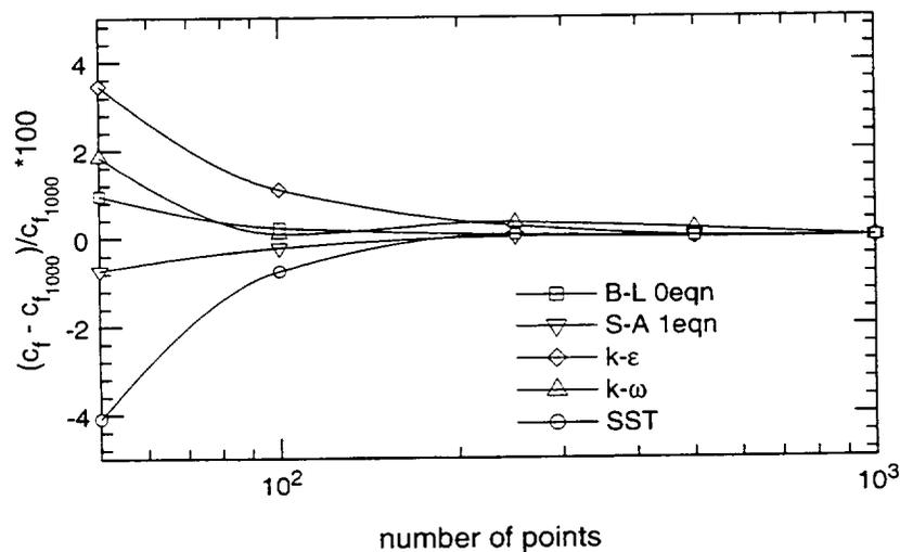
Figure 12.1. Grid sensitivity study—flat plate boundary layer.
