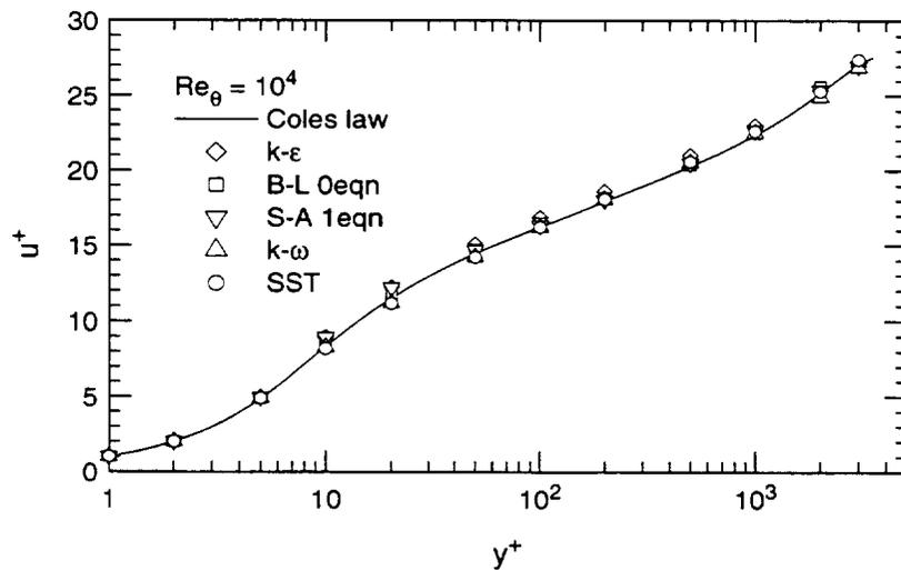
Figure 12.10. Comparison of the velocity profiles— $Re_\theta = 10^4$ .
