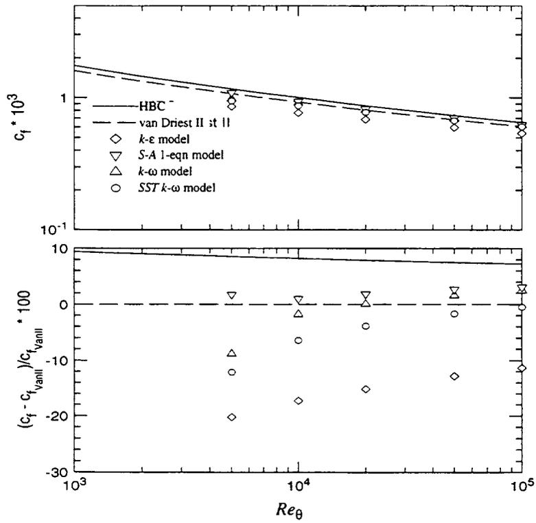
Figure 13.1. Comparison of the skin friction coefficients.
