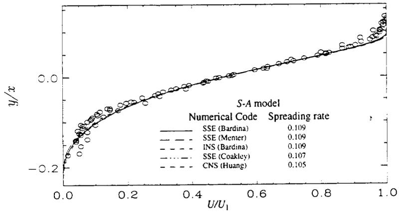
Figure 7.4. Comparison of code sensitivity in the prediction of the velocity profile for mixing layer flow.
