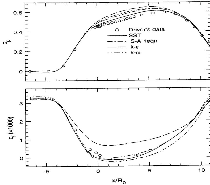
Figure 14.1. Comparison of surface pressure and skin friction coefficients.
