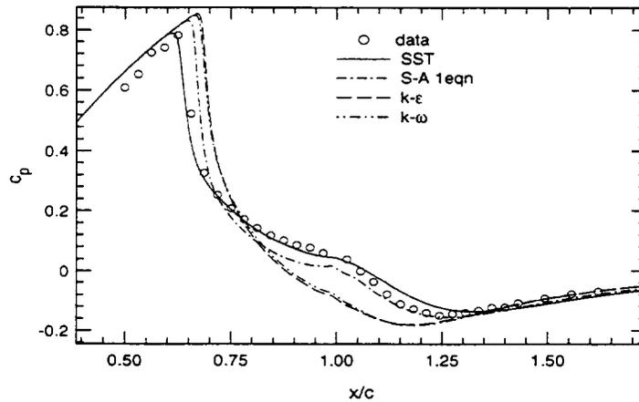
Figure 15.1. Comparison of surface pressure coefficient—transonic bump flow.
