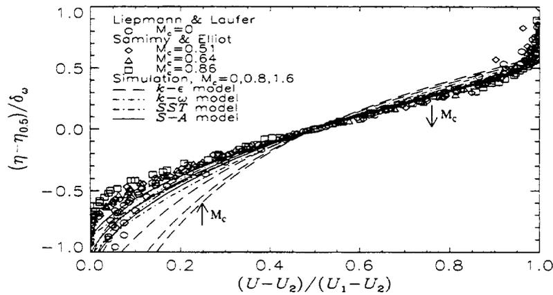
Figure 11.1. Comparison of velocity profiles for compressible mixing layer.
