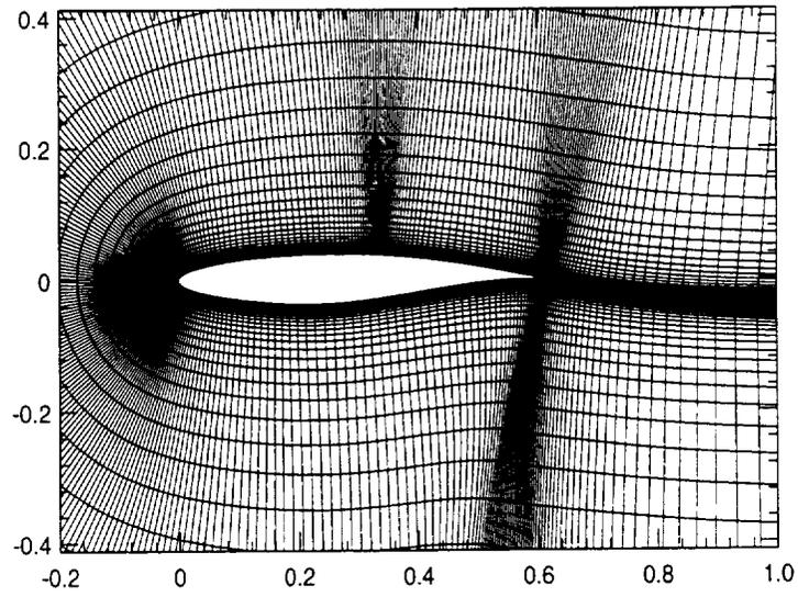
Figure 16.1. Computational grid with  $386 \times 82$  points.
