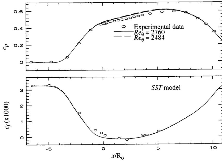
Figure 14.6. Effects of inlet boundary layer profiles.
