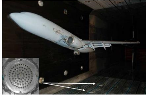
Figure 3: Boeing wind tunnel test using an Acoustic Phased Array mounted on the tunnel wall (Reproduced from Stoker et al., 2008).
