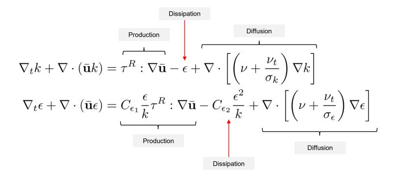
• The transport equation of the turbulence dissipation rate  $\epsilon$  used in this model can be derived by taking the following moment of the NSE equations,
