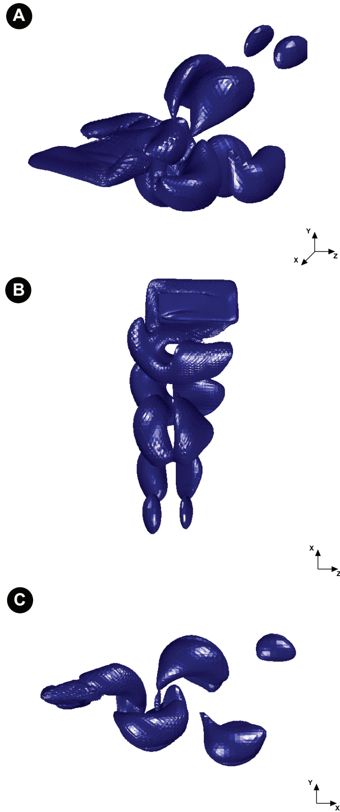
Figure 8.20: Vortex topology for the rolling wing case ( t=5.0 ). Flapping parameters: St = 0.25 , f_{roll} = 1.0 , Re = 500 . A) Perspective view. B) Top view. In this view the right wing-tip corresponds to the hinged extreme. C) Side view.
