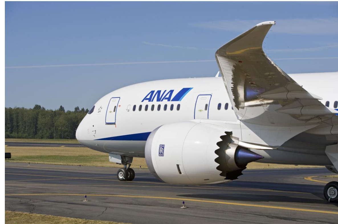
High lift devices (flaps and slats) and saw-teeth (chevrons) on engine nozzle
