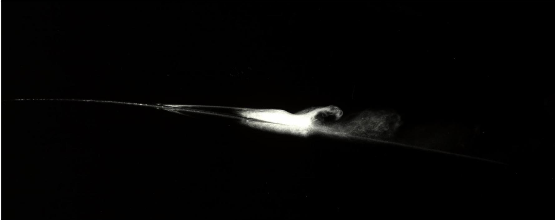
Smoke flow visualization of a laminar separation bubble on the Eppler 387 airfoil at a chord Reynolds number of 100 000 and 2 degrees angle of attack.
