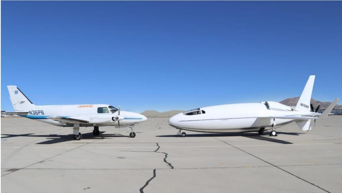
**Old vs. new:** Piper PA-31 (left aircraft) next to the Otto Celera 500L (right aircraft). Extensive use of laminar flow surfaces in the Otto Celera 500L results in approximately 59% reduction in drag compared to a similar sized conventional aircraft.
