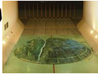
Figure 5 Terrain Model in Wind Tunnel
