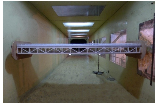
Figure 12 Section Model of Dimu River Bridge
