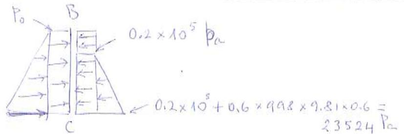
$$M_{\text{destra}} = 2 \times 10^4 \times 0.7 \times 0.35 + \frac{3524}{2} \times 0.6 \times \left( \frac{2}{3} \times 0.6 + 0.1 \right) = 5428.7 \text{ Nm}$$
