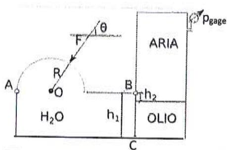
$$M_{\text{destra}} = 10^4 \times 0.8 \times 0.4 + 0.8 \times 998 \times 9.81 \times \frac{0.6}{2} \times 0.6 \times \left( \frac{2}{3} \times 0.6 + 0.2 \right)$$
