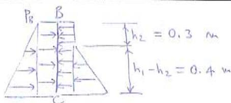
$$M_{\text{destra}} = 3 \times 10^4 \times 0.7 \times 0.35 + 0.6 \times 998 \times 9.81 \times 0.2 \times 0.4 \times \left( \frac{2}{3} \times 0.4 + 0.3 \right) = 7616 \text{ Nm}$$
