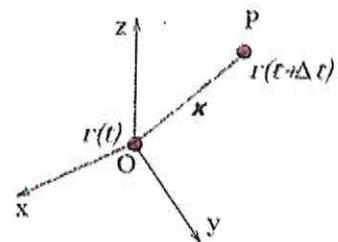
$$\underline{u}_P = \underline{u}_O + \nabla \underline{u} \big|_O \cdot \underline{x} = \underline{u}_O + \underline{\Omega} \cdot \underline{x} + \underline{E} \cdot \underline{x}$$
