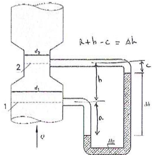
$$P_1 + \frac{1}{2} \rho v_1^2 = P_2 + \frac{1}{2} \rho v_2^2 + \rho g (z_2 - z_1) \quad v_2 = v_1 \frac{d_1^2}{d_2^2} \text{ (continuità)}$$
