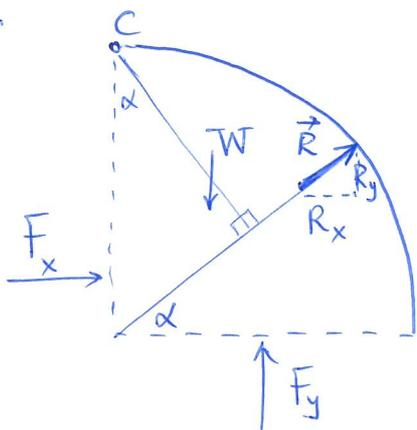
$$F_x = \left[ p_{\text{gage gas}} + \rho_1 g h_1 + \rho_2 g \left( h_2 + \frac{R}{2} \right) \right] \cdot R \cdot 1 = R_x$$
