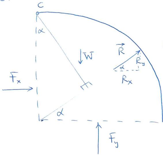
$$F_x = \left[ P_{\text{gage gas}} + \rho_1 g h_1 + \rho_2 g \left( h_2 + \frac{R}{2} \right) \right] \cdot R \cdot 1 = R_x$$
