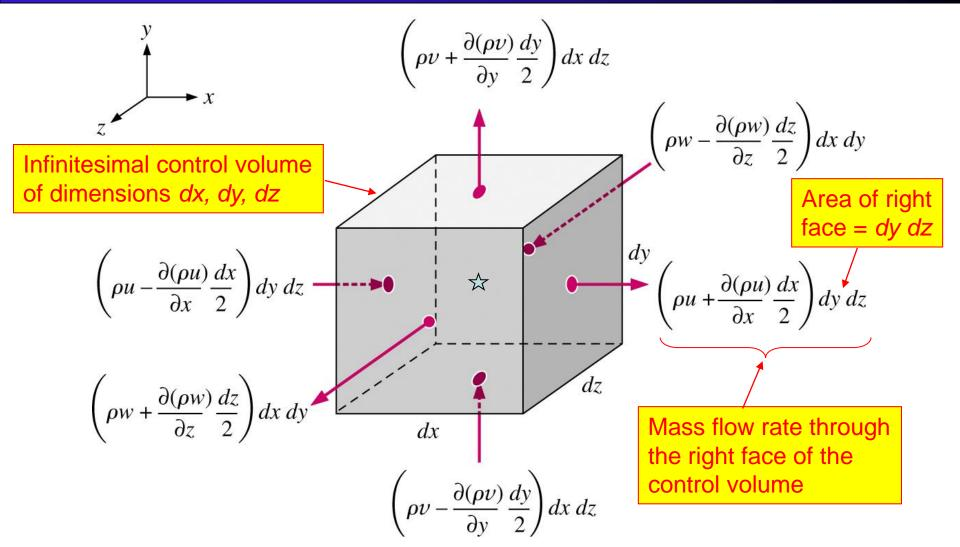
Now, sum up the mass flow rates into and out of the 6 faces of the CV
