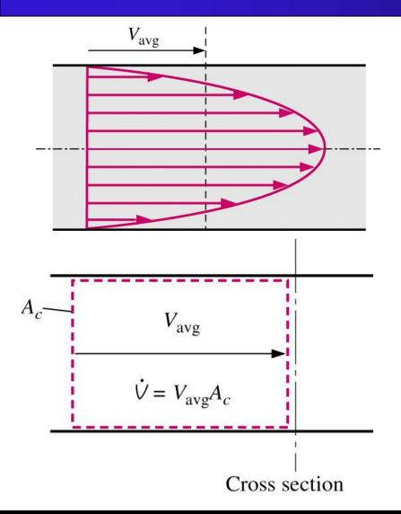
Integral in  $\dot{m}$  can be replaced with average values of  $\rho$  and  $V_n$
