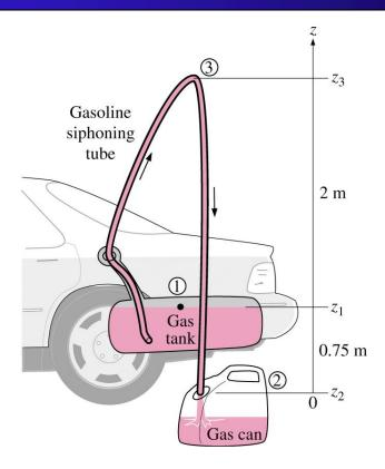
Siphon diameter = 4 mm;  $\rho_{gasoline}$  = 750 kg/m³; no frictional losses. Determine the time to siphon 4L of gasoline, and the pressure at point 3 (careful of cavitation at point 3!).
