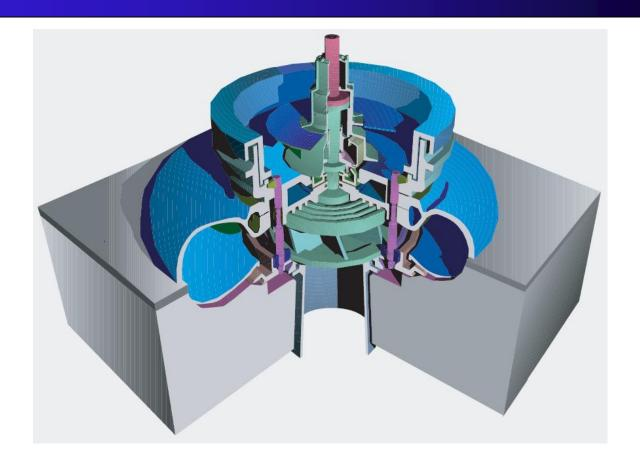
Distributor, Francis runner and shaft The choice of Francis, Kaplan or Pelton runners is based on the water mass flow rate and on the available "head".
