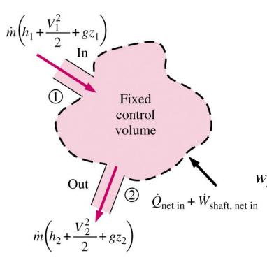
For single-stream devices, mass flow rate is constant. The steady flow energy equation per unit mass reads:
