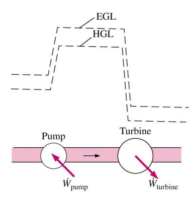
Steep jump (or drop) in EGL and HGL appear whenever mechanical energy is added to (or removed from) the fluid by a pump (or a turbine).
