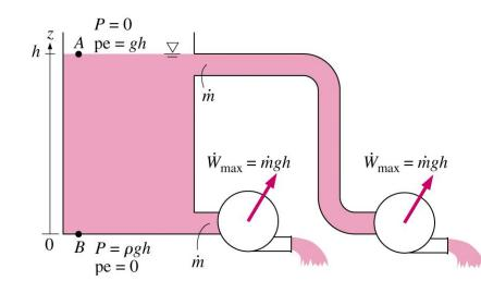
An ideal hydraulic turbine produces the same work per unit mass  $w_{turbine} = gh$  whether it receives water from the top or from the bottom of the container (in the absence of irreversible losses).
