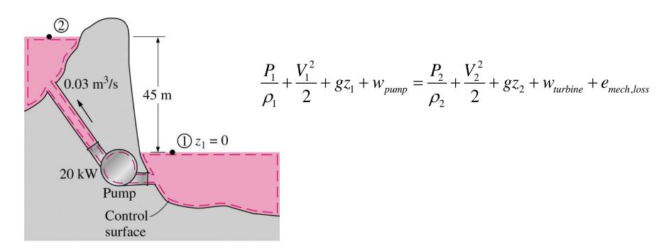
Determine the mechanical power lost (and the head loss  $h_L$ ) while pumping water to the upper reservoir.
