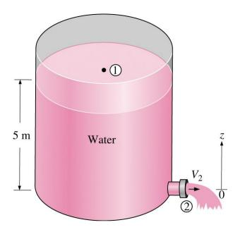
Flow irrotational and incompressible; flow quasi-steady (water drains slowly); no frictional losses nor flow disturbances. Exit velocity is given by  $V_2 = (2 \ g \ z_I)^{1/2}$  (Torricelli equation)
