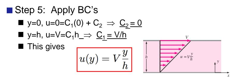
For pressure, no explicit BC, therefore  $C_3$  can remain an arbitrary constant (recall only  $\nabla P$  appears in NSE).
