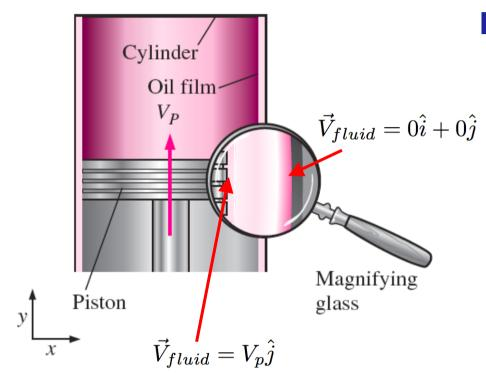
For a fluid in contact with a solid wall, the velocity of the fluid must equal that of the wall
