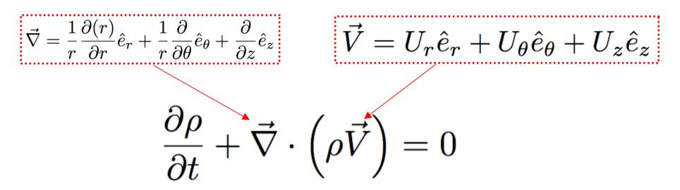
$$\frac{\partial \rho}{\partial t} + \frac{1}{r} \frac{\partial (r \rho U_r)}{\partial r} + \frac{1}{r} \frac{\partial (\rho U_\theta)}{\partial \theta} + \frac{\partial (\rho U_z)}{\partial z} = 0$$
