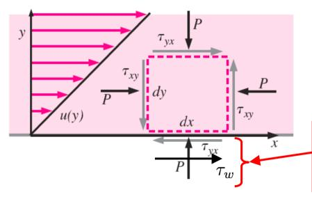
Shear force per unit area acting on the wall
