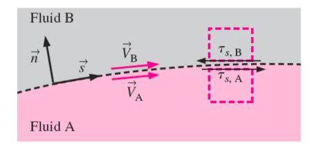
When two fluids meet at an interface, the velocity and shear stress must be the same on both sides
