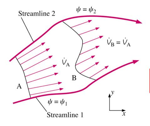
Difference in  $\psi$  between streamlines is equal to volume flow rate between streamlines
