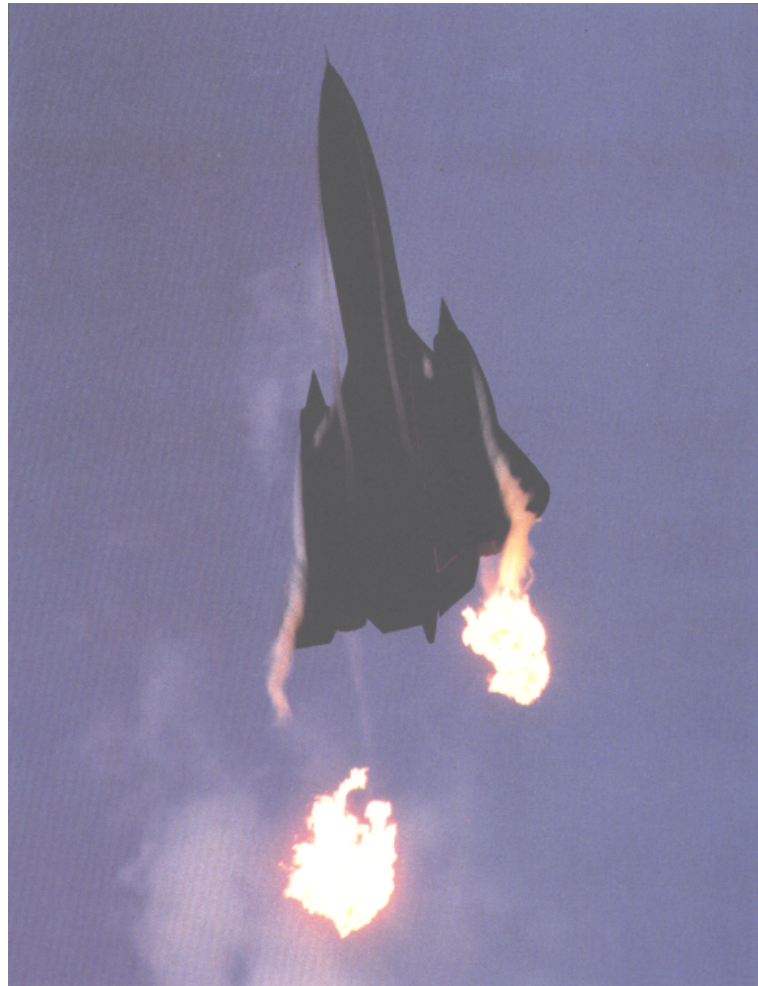
Figure 1.11: Flame blow-off in the SR-71 during a high-acceleration manoeuvre [5].
