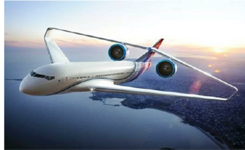
(b) Semi-conventional aircraft (Box wing aircraft [10]).
