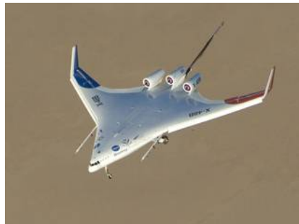
(e) Blended wing Body concept ( www.nasa.gov/centers/dryden/research/X-48B ).
