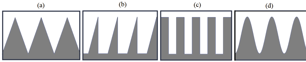
Figure 1.3: (a): Triangular grooves; (b): Saw-tooth grooves; (c): Rectangular grooves; (d): Sinusoidal grooves.
