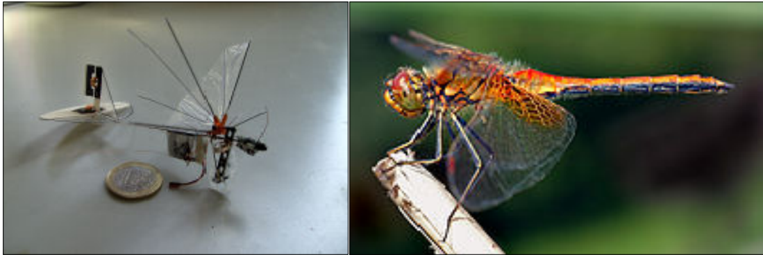
Figure 1.2: Left: The Delfly Micro, a very small remote-controlled aircraft with camera, weighing just 3 grams and measuring 10 cm (Source - http://www.delfly.nl/?site=DIII&menu=home&lang=en , website of Delfly project, TU Delft). Right: The dragonfly Yellow-winged Darter , inspiration behind the Delfly Micro (Source - http://en.wikipedia.org/wiki/Dragonfly ).
