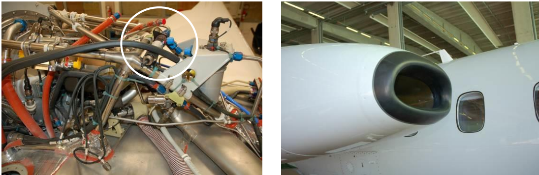
Fig.2.6 Distributor/Vacuum valve e boot gonfiabile
