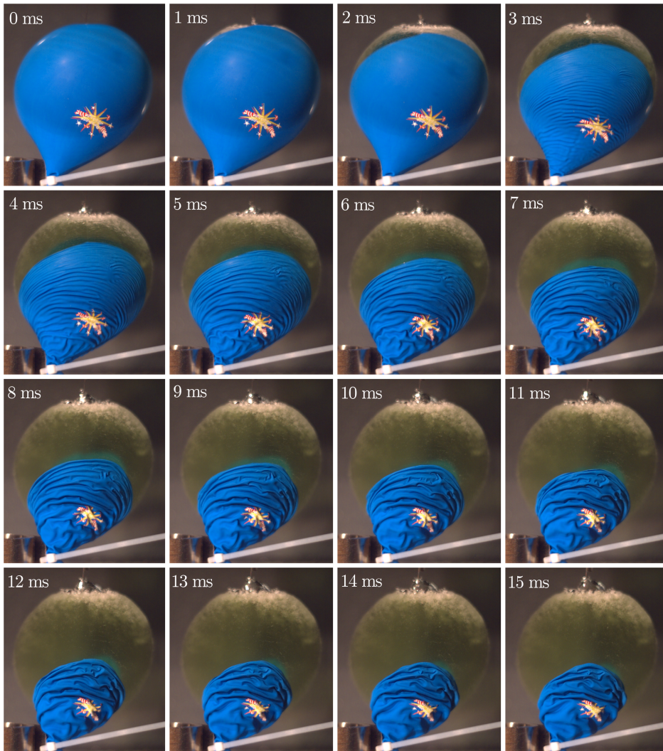
Figure 7.4: Underwater explosion of a balloon filled with a mixture of water and green colorant. The balloon is anchored at the bottom of the tank in which it is immersed.
