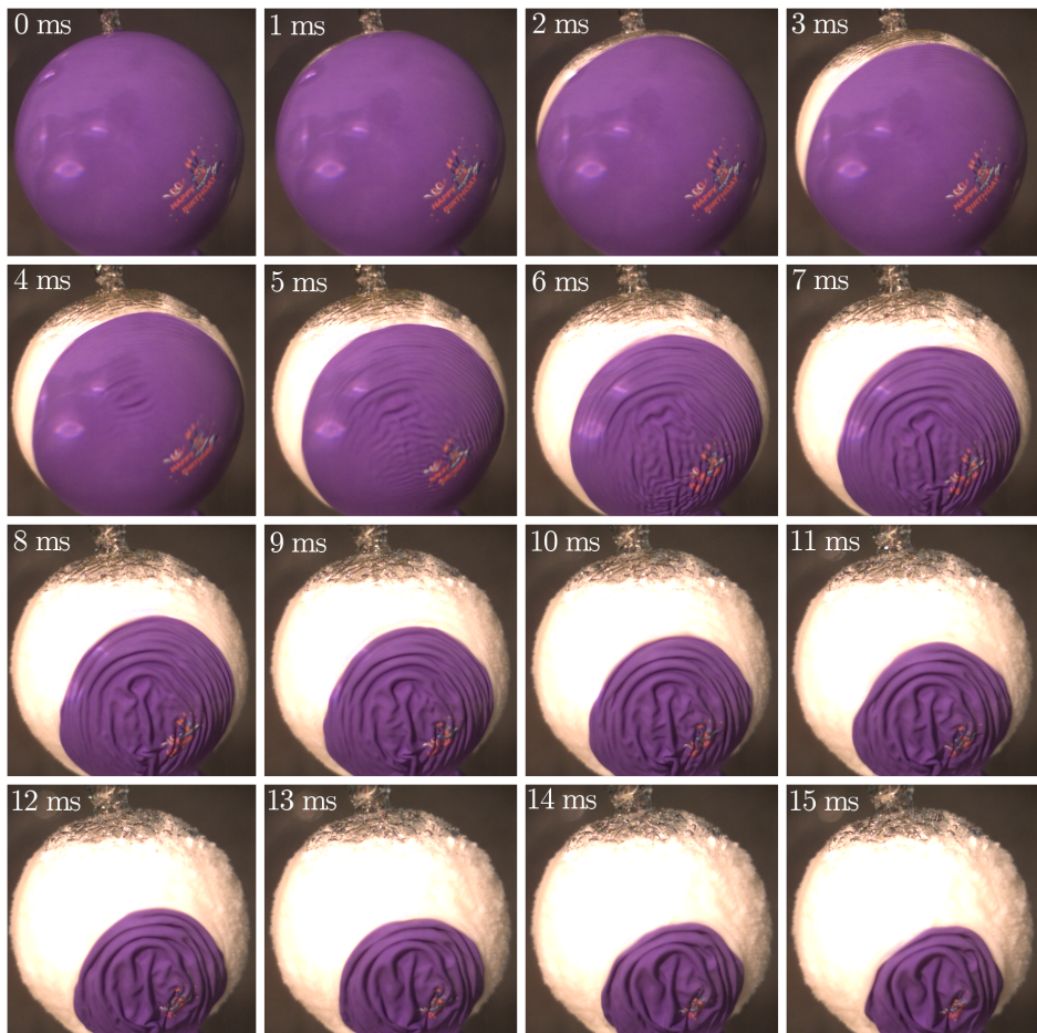
Figure 7.5: Underwater explosion of a balloon filled with water mixed with milk powder. The balloon is anchored at the bottom of the tank in which it is immersed
