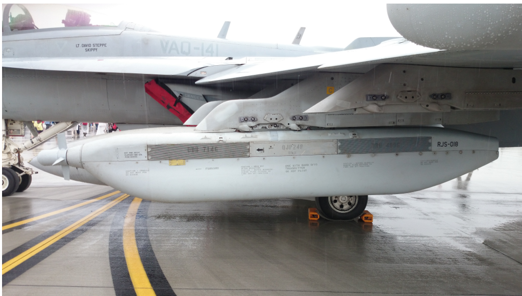
Fig. 3.1: AN/ALQ-99 electronic-warfare pod mounted under a Boeing E/A-18G's wing. The RAT can be seen at the front of the device. Wikimedia Commons
