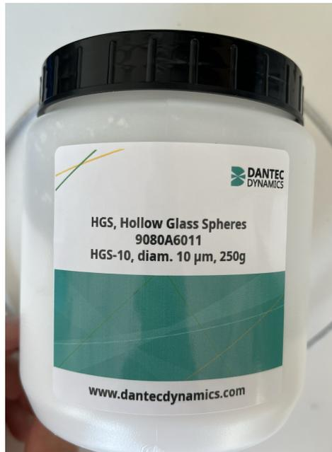
Figura 3.14: HGS  $1.1\text{g}/\text{cm}^3$   $\phi=10\ \mu\text{m}$
