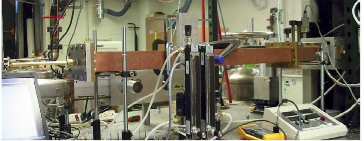
Laminar flame burner coupled to a rectangular microwave cavity operating in the TE_{01n} resonant mode. The cavity is formed from WR430 rectangular waveguide with an adjustable short forming one end wall and a 3-stub tuner forming a partially reflecting wall on the other end. The photo shows the actual laboratory set-up.
