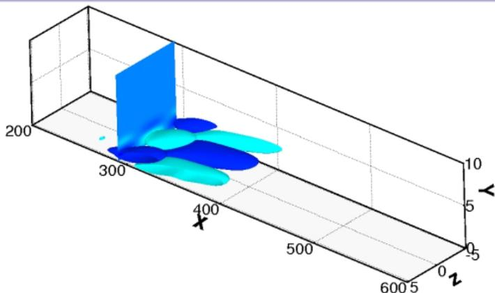
**Superposition of local optimals and suboptimals at different  $\alpha$  → the global optimal perturbation is qualitatively recovered**
