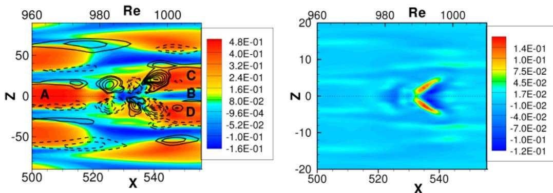
**Figure:** Streamwise (a) and wall-normal (b) perturbation at  $T = 220$ . The solid and dashed lines represent positive and negative spanwise velocities.
