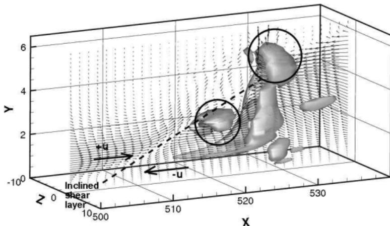
**Figure:** Iso-surfaces of the  $Q$  criterion and  $u, v, w$  vectors on the  $x - y$  plane at  $z = 0$  at  $t = 180$ .
