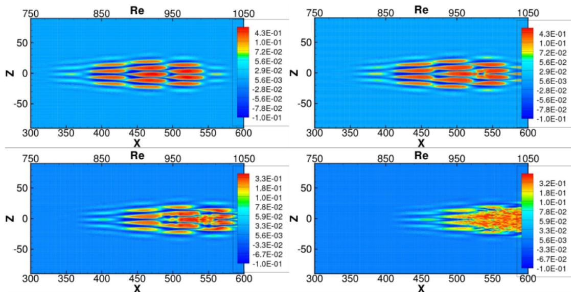
Streamwise velocity contours at  $y = 1$  and  $E_0 = 0.5$  at four times:
