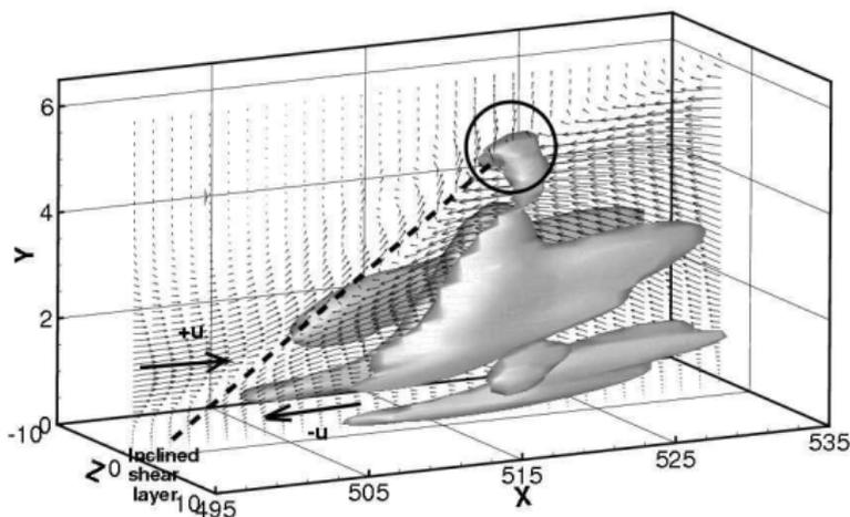
**Figure:** Iso-surfaces of the  $Q$  criterion and  $u, v, w$  vectors on the  $x - y$  plane at  $z = 0$  at  $t = 165$ .
