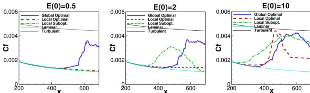
**Figure:** Mean skin friction factor of the considered flow perturbed with global, local, and sub-optimal disturbances, for from left to right  $E_0 = 0.5$ ,  $E_0 = 2$  and  $E_0 = 10$ .
