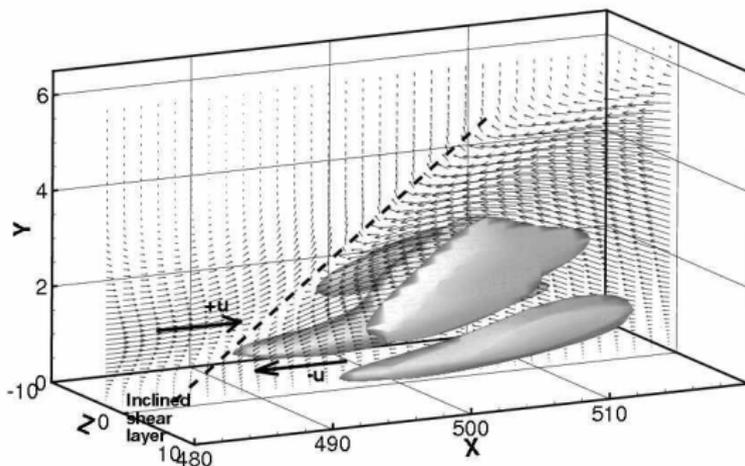
**Figure:** Iso-surfaces of the Q criterion and  $u, v, w$  vectors on the  $x - y$  plane at  $z = 0$  at  $t = 145$ .
