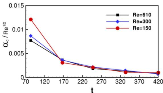
**The characteristic wavenumber is found to increase approximately with the square root of  $Re \rightarrow$  the curves of  $\alpha_c$  normalized with  $\sqrt{Re}$  collapse onto one for sufficiently large times**
