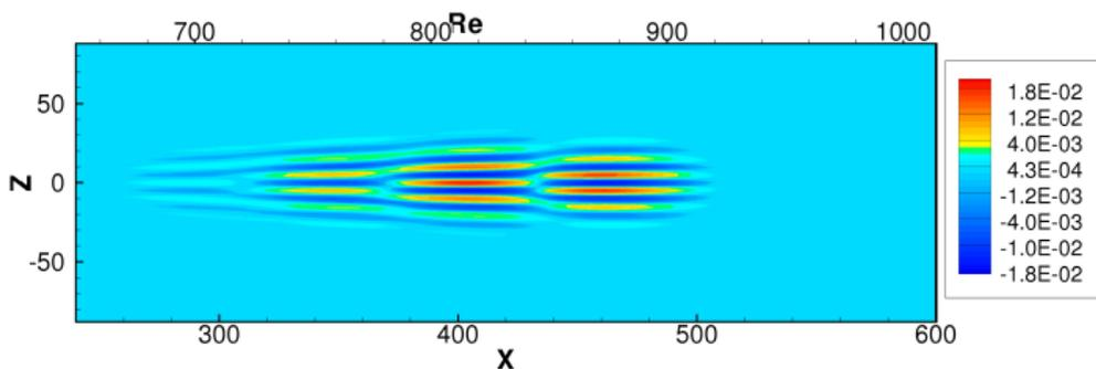
Figure: Streamwise near-optimal perturbation at  $t = 0$ ,  $y = 1$ .
