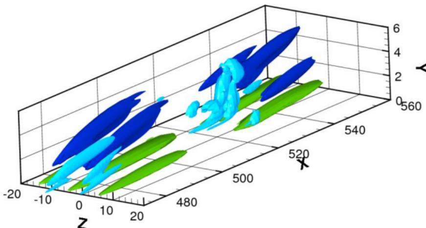
**Figure:** Iso-surfaces of negative (blue) and positive (green) streamwise perturbations, and Q-criterion surfaces (light blue).
