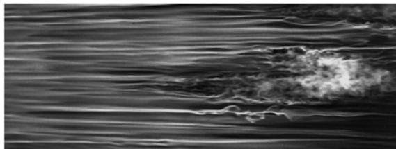
**Figure:** Wind tunnel smoke visualization of transition in a boundary layer subjected to free stream turbulence (KTH, Stockholm).
