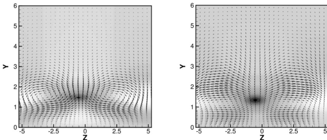
**Figure:** Optimal perturbation at  $t = 0$  and  $t = t_{max}$  for  $Re = 610$ . Vectors represent the wall-normal and spanwise velocity components, shades of grey are relative to the streamwise velocity.
