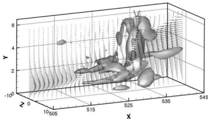
**Figure:** Iso-surfaces of the  $Q$  criterion and  $u, v, w$  vectors on the  $x - y$  plane at  $z = 0$  at  $t = 190$ .
