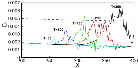
FIG. 5. (Color online) Streamwise distribution of the spanwise-averaged skin-friction coefficient for  $T=50, 100, 150, 200, 250$  (solid lines from left to right) together with the laminar and turbulent theoretical distributions (bottom and top dashed lines, respectively).
