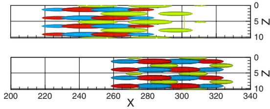
FIG. 3. (Color online) Isosurfaces of the velocity components of the perturbation obtained by the linear optimization for the target time  $T=75$ , for an initial energy  $E_0=0.01$ . Light gray (green) indicates the streamwise component ( $u=-0.00015$  at  $t=0$  and  $u=-0.1$  at  $t=75$ ); gray (blue) and black (red) indicate negative and positive spanwise components, respectively ( $w=\pm 0.004$  at  $t=0$  and  $w=\pm 0.01$  at  $t=75$ ). Axes are not in the same scale.
