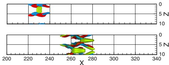
FIG. 4. (Color online) Isosurfaces of the velocity components of the perturbation obtained by the nonlinear optimization for the target time  $T=75$ , for an initial energy  $E_0=0.01$ . Light gray (green) indicates the streamwise component ( $u=-0.01$  at  $t=0$  and  $u=-0.1$  at  $t=75$ ); gray (blue) and black (red) indicate negative and positive spanwise components, respectively ( $w=\pm 0.007$  at  $t=0$  and  $w=\pm 0.05$  at  $t=75$ ). Axes are not in the same scale.
