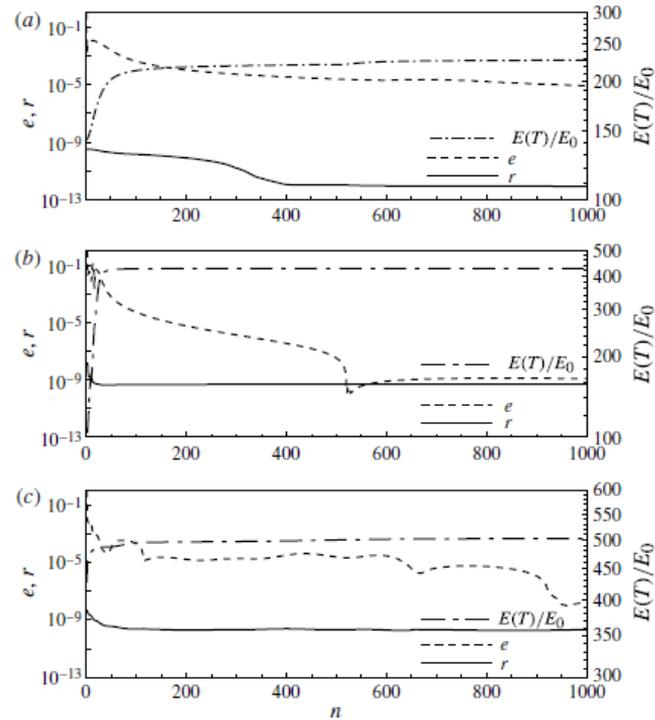
FIGURE 1. Convergence history for a nonlinear optimization at target time (a)  $T = 50$  with  $E_0 = 0.005$ , (b)  $T = 30$  with  $E_0 = 0.025$ , and (c)  $T = 30$  with  $E_0 = 0.1$ . Solid line, residual; dashed line, error on the objective function; dot-dashed line, value of the energy gain.
