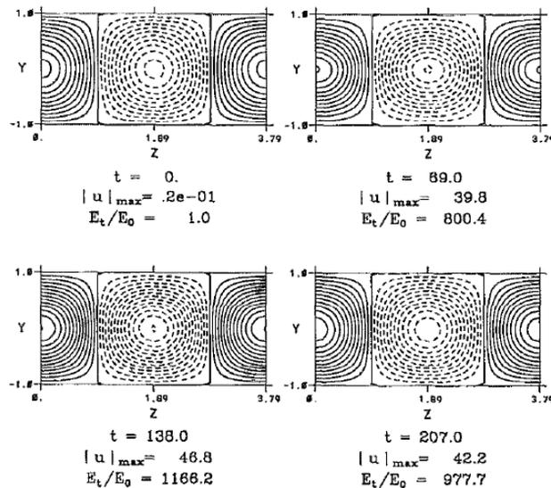
FIG. 4. Development of the perturbation streamwise velocity  $u$  for the best growing perturbation independent of  $x$  in Couette flow with  $R = 1000$ , located at  $\beta = 1.66$ ,  $\tau = 138$ . Values are normalized by the maximum value of  $v$  at time  $t=0$ .
