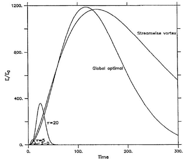
FIG. 8. Energy growth versus time for the global optimal, the streamwise vortex, and 2-D perturbation which grow the most, and perturbations which grow the most in 5 and 20 advective time units in Couette flow with  $R = 1000$ .
