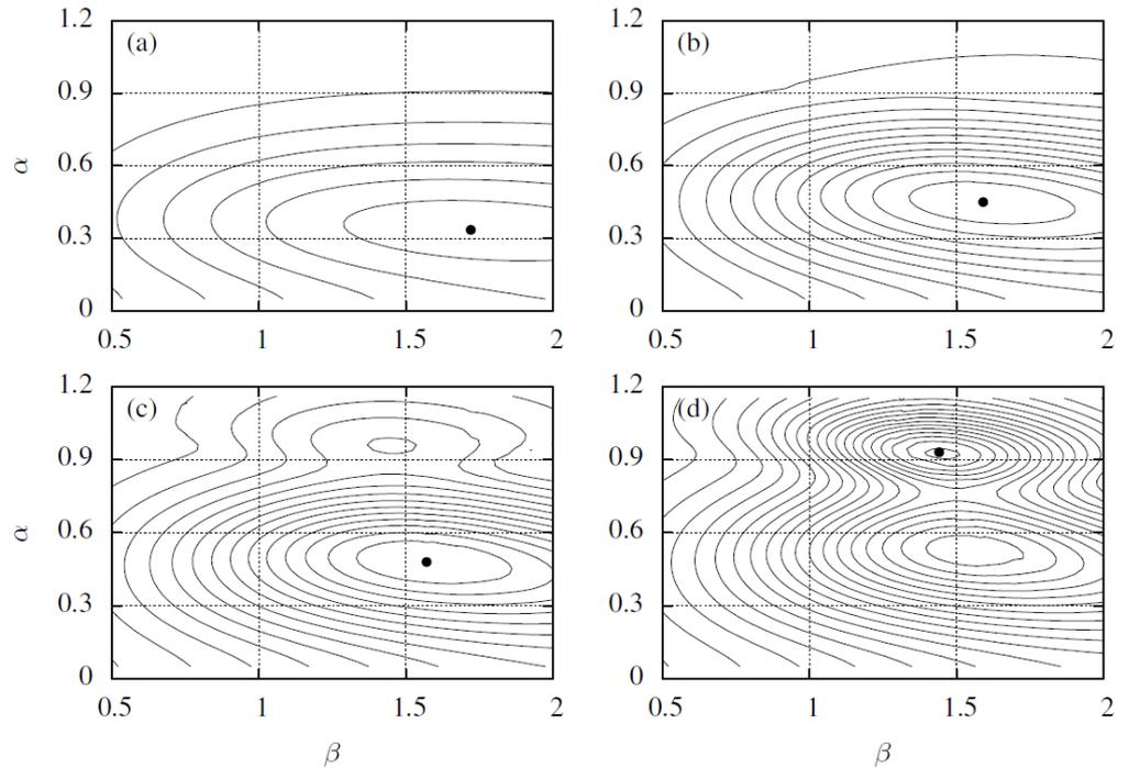
FIGURE 6. Gain  $G$  in the  $\alpha - \beta$  plane for  $Re = 400$  and  $T = 20$ ; (a)  $\epsilon \rightarrow 0$  with contour values from 20 to 120, (b)  $\epsilon = 0.0145$  with contour values from 20 to 240, (c)  $\epsilon = 0.0153$  with contour values from 20 to 300, (d)  $\epsilon = 0.01603$  with contour values from 20 to 380. The interval among adjacent isolines is  $\Delta G=20$  in frames. The maximum value of  $G$  for each  $\epsilon$  is denoted by a filled circle.
