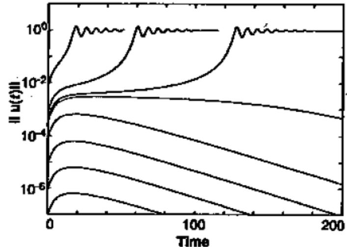
**Fig. 10.**  $\|\mathbf{u}(t)\|$  for solutions to the nonlinear  $2 \times 2$  model problem of Eq. 14 with initial amplitudes  $\|\mathbf{u}(0)\| = 10^{-7}, 10^{-6}, 10^{-5}, 10^{-4}, 4 \times 10^{-4}, 5 \times 10^{-4}, 10^{-3},$  and  $10^{-2}$ . The threshold amplitude is  $\|\mathbf{u}(0)\| = 4.22 \times 10^{-4}$ .
