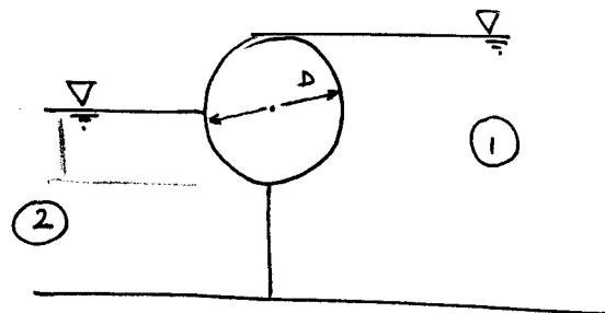
$$F_o |_{\text{lato fluido } 2} = \gamma_2 \frac{\pi (\frac{D}{2})^2}{2} h_{\text{baricentro}} \text{ semi cerchio}$$
