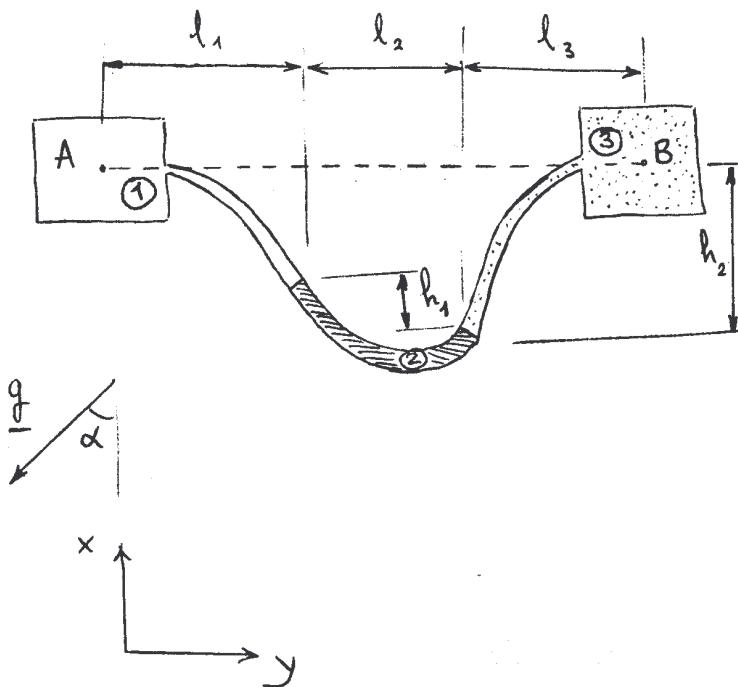
$$\begin{aligned}\alpha &= \pi/4 \\ p_B &= 200 [\text{kPa}] \\ l_1 &= l_2 = l_3 = 1 [\text{m}] \\ h_1 &= 30 [\text{cm}] \\ h_2 &= 40 [\text{cm}] \\ \rho_1 &= 1000 [\text{kg m}^{-3}] \\ \rho_2 &= 3000 [\text{kg m}^{-3}] \\ \rho_3 &= 1500 [\text{kg m}^{-3}]\end{aligned}$$
