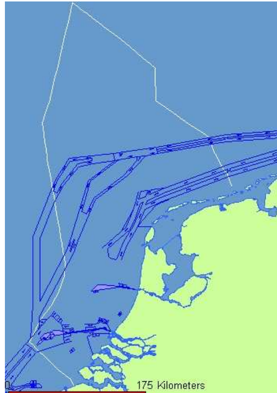
Figure 10: Navigation channels present in the North Sea along the Dutch coast. Approximately 500,000 ships travel along these paths. More than 220,000 run through the channel leading to the Europort of Rotterdam (source: Noordzeeatlas).
