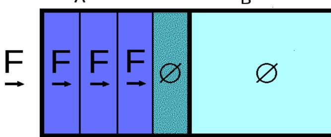
**Example of shadow**: obstacles at the border between cells A and B project their shadow towards cell B.
