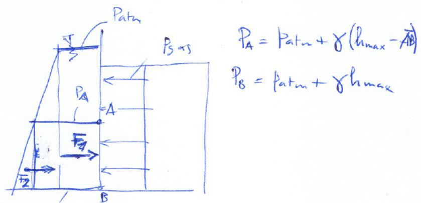
$$F_1 = P_A \cdot \overline{AB} \cdot L = [P_{\text{atm}} + \gamma(h_{\text{max}} - \overline{AB})] \overline{AB} \cdot L = \\ = [10^5 + 780.981(h_{\text{max}} - 1)] \cdot 1 \cdot 1 = 100000 + 780.981h_{\text{max}} - 780.981 = 780.981h_{\text{max}} + 92348 \text{ N}$$
